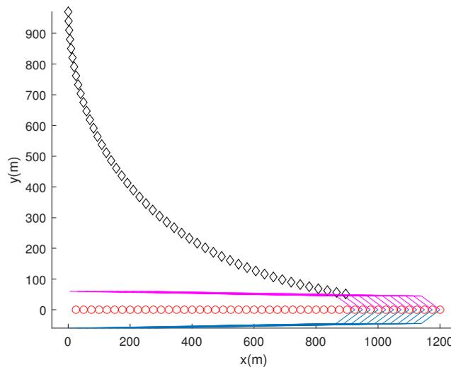
**Figure 4.** An illustration of the target ship’s wake as the ship moves with a constant velocity ([5,0] in m/s) starting from the origin. Blue line segments represent the right wake, and magenta line segments represent the left wake. Red circles indicate the ship’s trajectory every 5 s. Black diamonds depict the AUV’s trajectory every 5 s.
