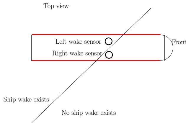
**Figure 2.** The top view of the AUV. The two circles in this figure represent the two wake sensors. In addition, the AUV has flank array sonar (bold red line segments) attached to either side. The slanted line indicates the boundary of the target ship’s wake.
