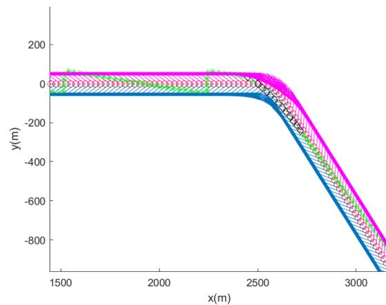
**Figure 10.** Scenario 2. Enlarged version of Figure 9 for improved visibility. Blue line segments represent the target ship’s wake to the ship’s right, and magenta line segments represent the target ship’s wake to the ship’s left. Red circles indicate the ship’s trajectory every 5 s. Black diamonds represent the AUV’s trajectory as the AUV applies target bearing angle measurements. Green asterisks show the AUV’s trajectory as the AUV does not use target bearing angle measurements.
