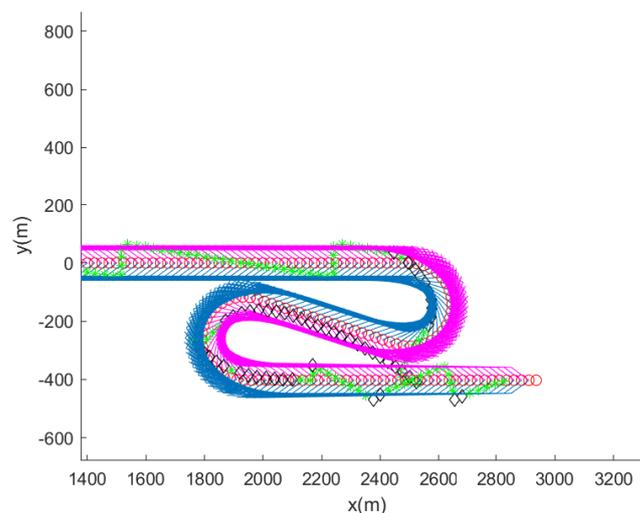
**Figure 16.** Scenario 5. Enlarged version of Figure 15 for improved visibility. Blue line segments represent the target ship's wake to the ship's right, and magenta line segments represent the target ship's wake to the ship's left. Black diamonds represent the AUV's trajectory as the AUV applies target bearing angle measurements. Green asterisks show the AUV's trajectory as the AUV does not use target bearing angle measurements. Red circles indicate the ship's trajectory every 5 s.
