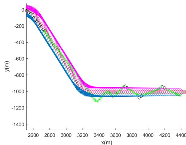
**Figure 12.** Scenario 3. Enlarged version of Figure 11 for improved visibility. Blue line segments represent the target ship’s wake to the ship’s right, and magenta line segments represent the target ship’s wake to the ship’s left. Red circles indicate the ship’s trajectory every 5 s. Black diamonds represent the AUV’s trajectory as the AUV applies target bearing angle measurements. Green asterisks show the AUV’s trajectory as the AUV does not use target bearing angle measurements.
