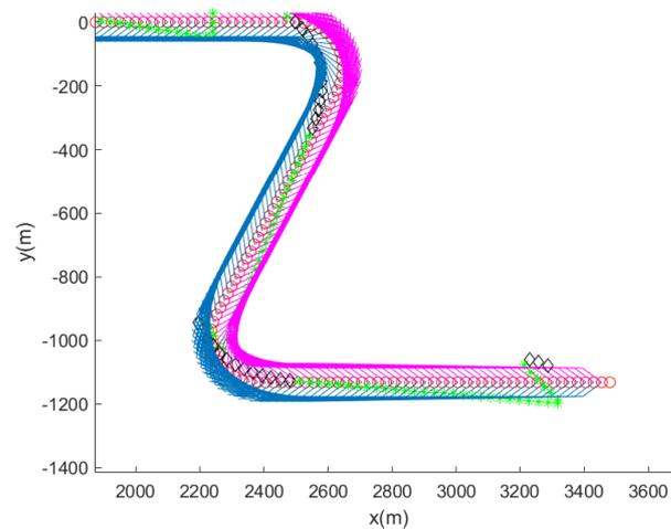
**Figure 14.** Scenario 4. Enlarged version of Figure 13 for improved visibility. Blue line segments represent the target ship’s wake to the ship’s right, and magenta line segments represent the target ship’s wake to the ship’s left. Black diamonds represent the AUV’s trajectory as the AUV applies target bearing angle measurements. Green asterisks show the AUV’s trajectory as the AUV does not use target bearing angle measurements. Red circles indicate the ship’s trajectory every 5 s.
