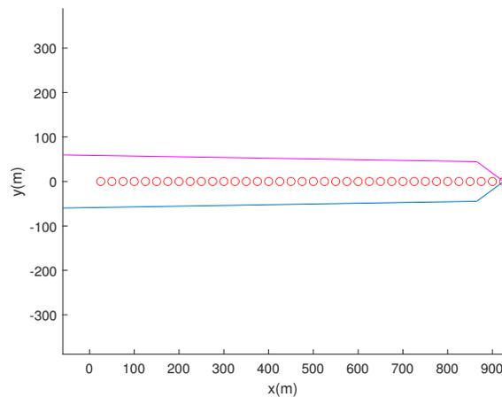
**Figure 1.** An illustration of the target ship’s wake as the ship moves with a constant velocity ( $[5,0]$  in m/s) starting from the origin. Blue line segments represent the target ship’s wake to the ship’s right, and magenta line segments represent the target ship’s wake to the ship’s left. Red circles indicate the ship’s trajectory every 5 s.
