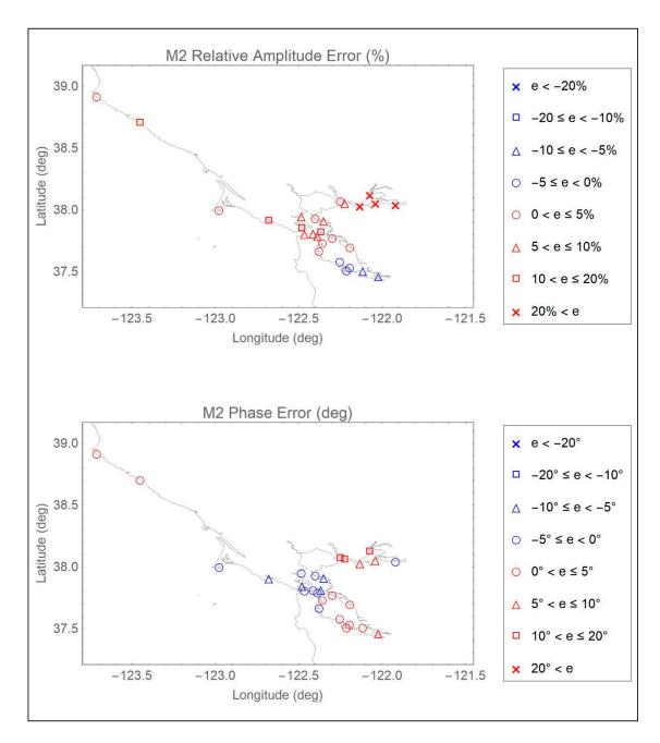
**Figure A16.** Distribution of ENPAC15 relative amplitude (%) and absolute phase (deg) errors for the  $M_2$  constituent: San Francisco Bay view.
