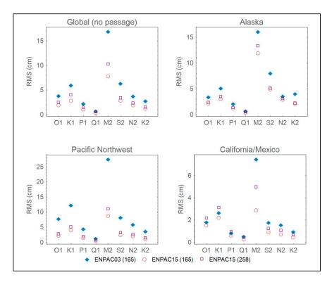
**Figure 9.** Mean root mean square errors (cm) in harmonic constituents for the ENPAC03 and ENPAC15 ADCIRC tidal databases for each region of the ENPAC model domain (note that the scale is not the same for each region).
