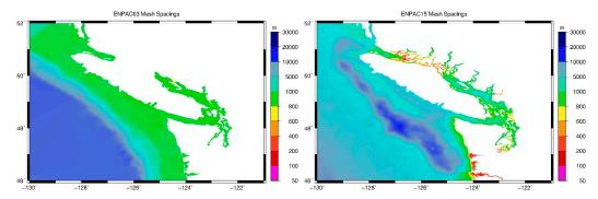
**Figure 4.** Comparison of coastal resolution in the ENPAC03 (left panel) and ENPAC15 (right panel) models for the Vancouver Island and Washington coast regions.
