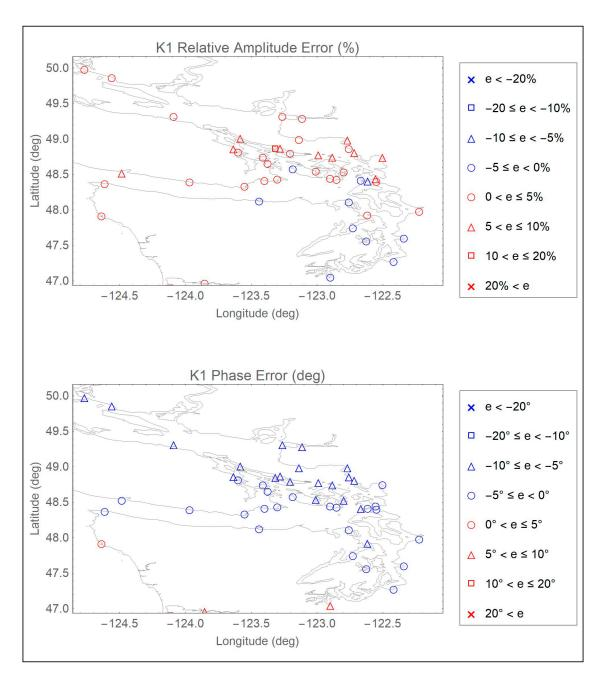
**Figure A20.** Distribution of ENPAC15 relative amplitude (%) and absolute phase (deg) errors for the  $K_1$  constituent: Puget Sound view.
