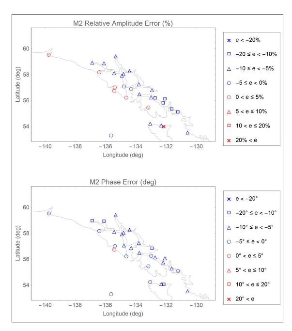
**Figure A23.** Distribution of ENPAC15 relative amplitude (%) and absolute phase (deg) errors for the  $M_2$  constituent: Southeast Alaska view.
