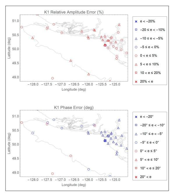
**Figure A22.** Distribution of ENPAC15 relative amplitude (%) and absolute phase (deg) errors for the  $K_1$  constituent: British Columbia coast view.
