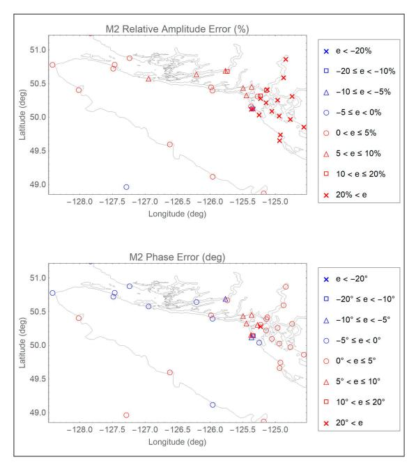
**Figure A21.** Distribution of ENPAC15 relative amplitude (%) and absolute phase (deg) errors for the  $M_2$  constituent: British Columbia coast view.
