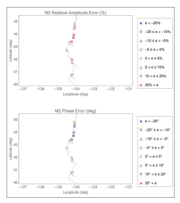
**Figure A17.** Distribution of ENPAC15 relative amplitude (%) and absolute phase (deg) errors for the  $M_2$  constituent: Northern California coast view.
