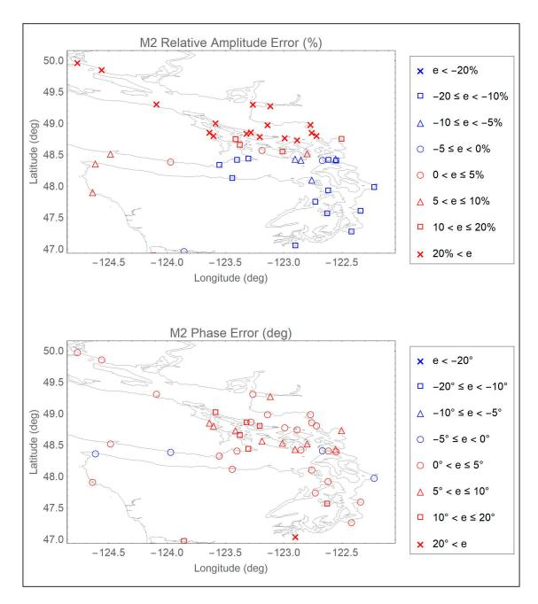
**Figure A19.** Distribution of ENPAC15 relative amplitude (%) and absolute phase (deg) errors for the  $M_2$  constituent: Puget Sound view.
