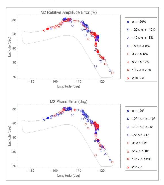
**Figure 10.** Relative amplitude (%) and absolute phase errors (deg) in the  $M_2$  constituent at each of the 258 global validation stations for the ENPAC15 database. Zoomed views are provided in Appendix D.
