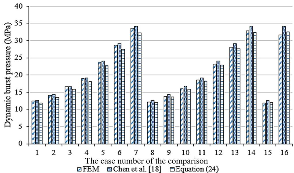
Figure 9. Comparisons between the FEM results and Equation (24), when  $t_d = 3.9$  ms.
