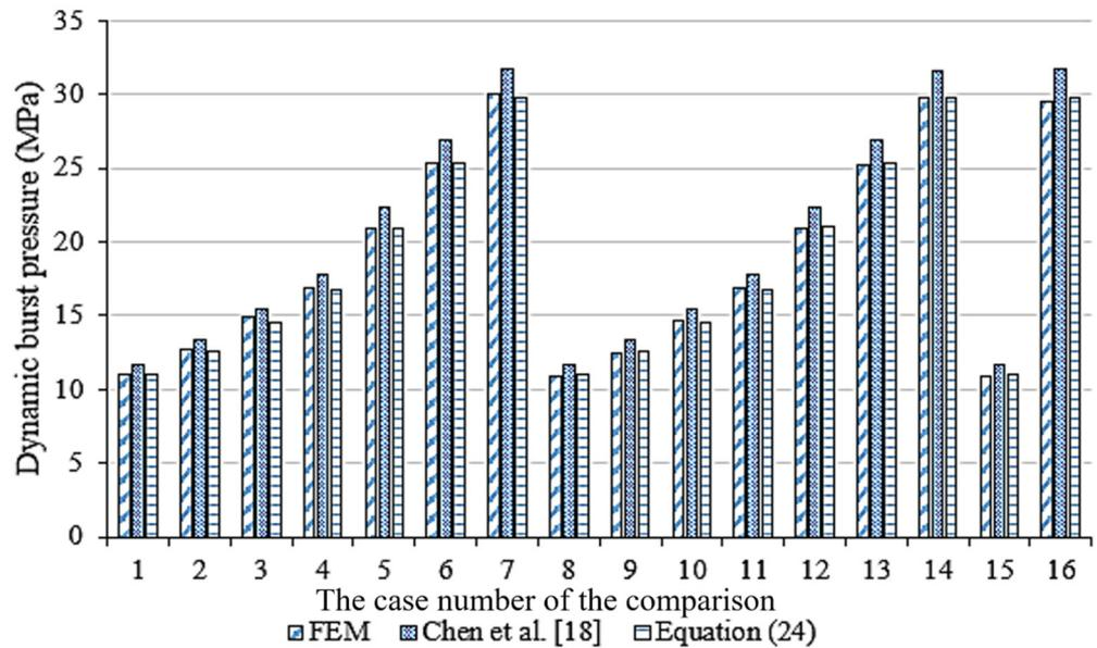
Figure 10. Comparisons between the FEM results and Equation (24), when  $t_d = 39$  ms.
