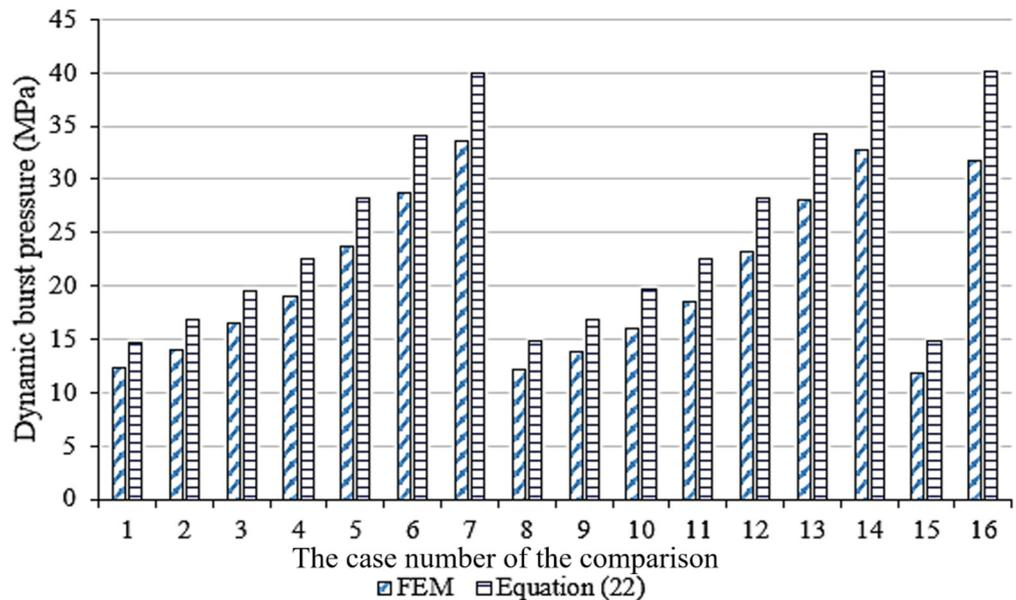
Figure 6. Comparisons between the FEM results and Equation (22), when  $t_d = 3.9$  ms.
