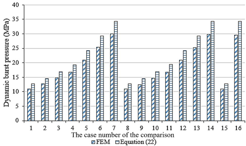
Figure 7. Comparisons between the FEM results and Equation (22), when  $t_d = 39$  ms.
