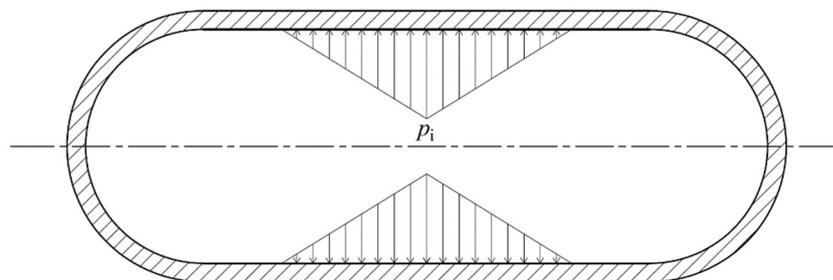
Figure 1. Geometrical model of a cylindrical shell subjected to a spindle-shaped load.
