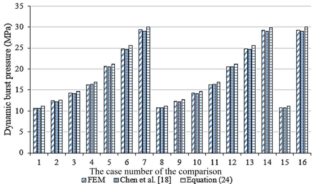
Figure 11. Comparisons between the FEM results and Equation (24), when  $t_d = 390$  ms.
