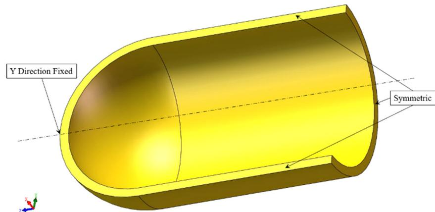
**Figure 4.** Boundary conditions of the finite element model.
