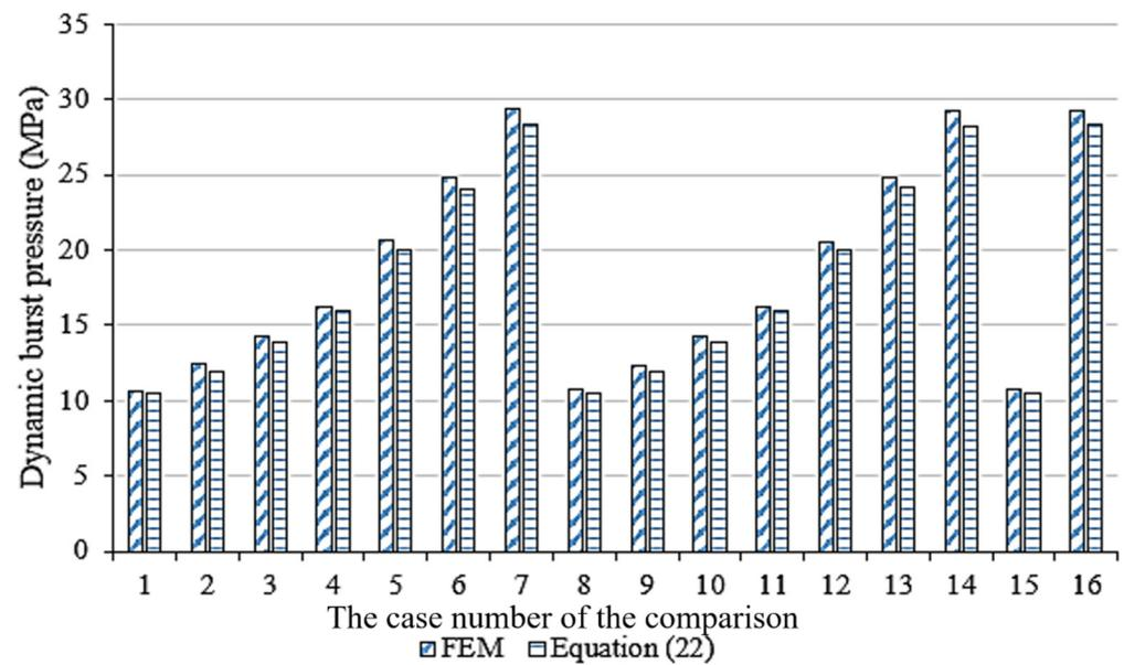
Figure 8. Comparisons between the FEM results and Equation (22), when  $t_d = 390$  ms.
