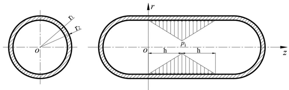
Figure 2. Model of a cylindrical shell and its spindle-shaped loadings.
