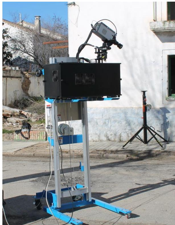
**Figure 4.** The LIF sensor operating in the field. It is placed on a manual mobile elevator for easy deployment.
