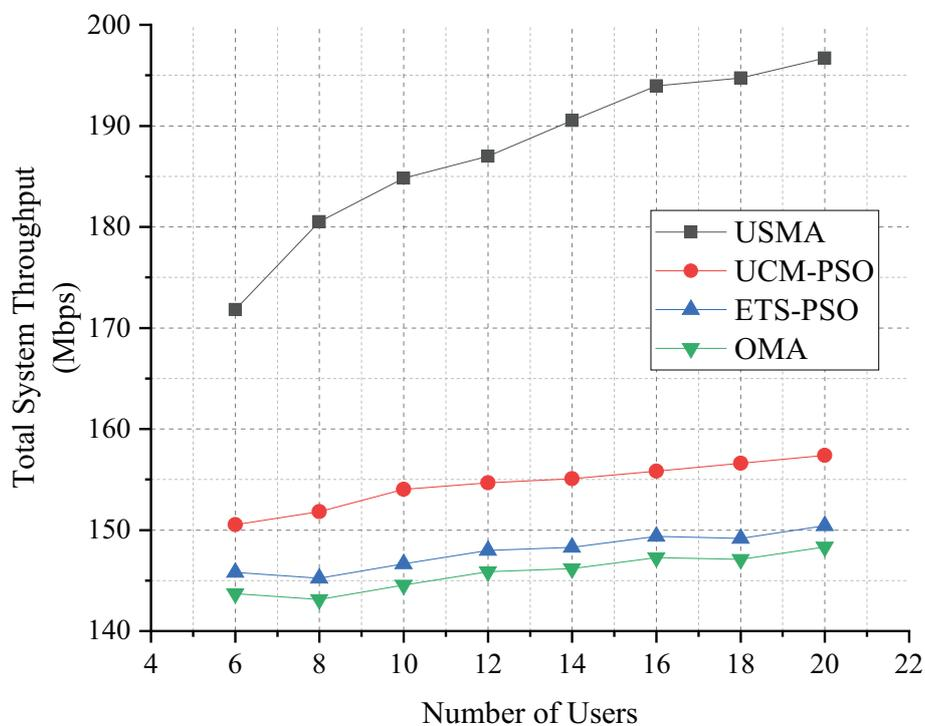
Figure 4. Achieved system throughput for  $S = 128$  channels, when the number of users ranges from 6 to 20.
