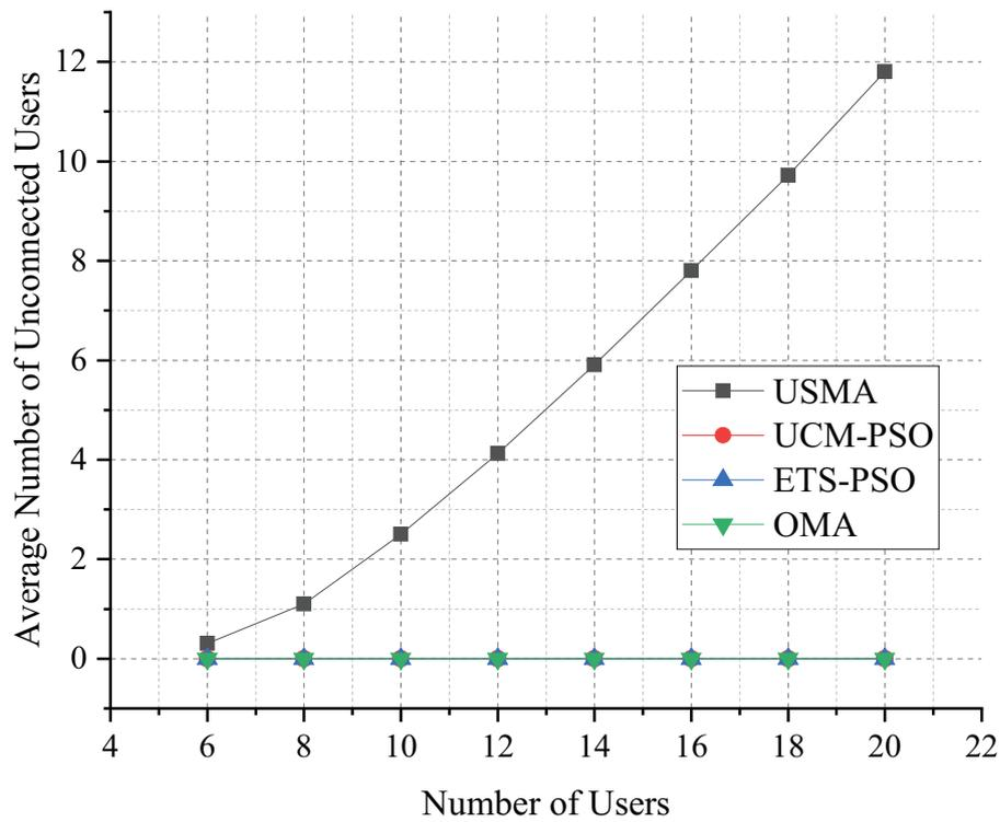
Figure 8. Average number of unconnected users for  $S = 128$  channels, when the number of users ranges from 6 to 20.
