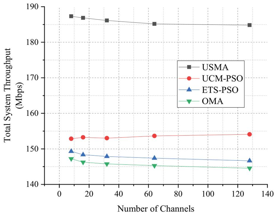
Figure 3. Achieved system throughput for  $K = 10$  users, when the number of channel ranges from 8 to 128.
