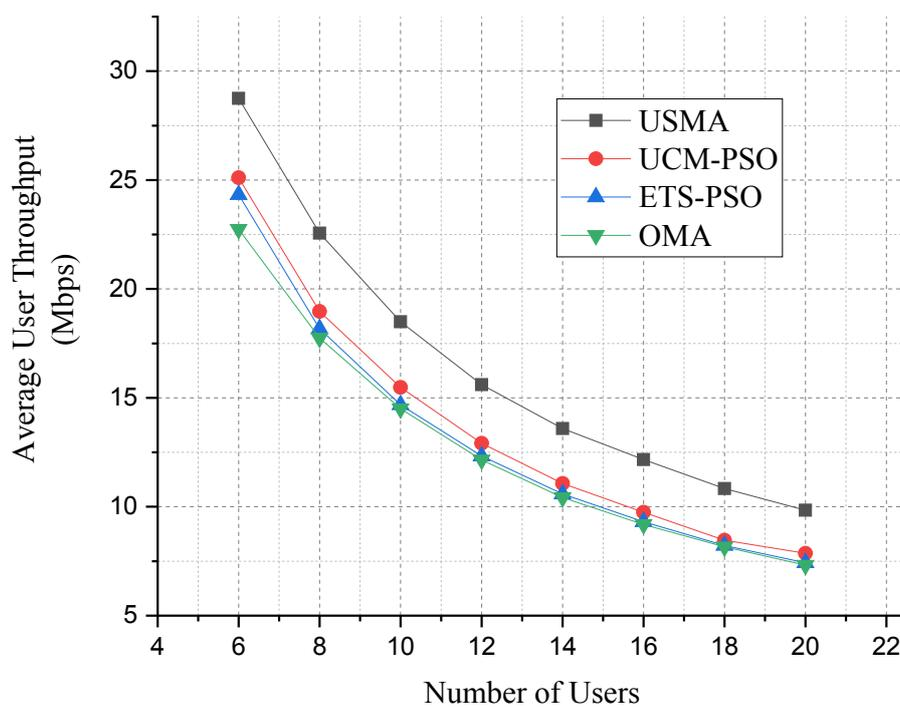
Figure 9. Average user throughput for  $S = 128$  channels, when the number of users ranges from 6 to 20.
