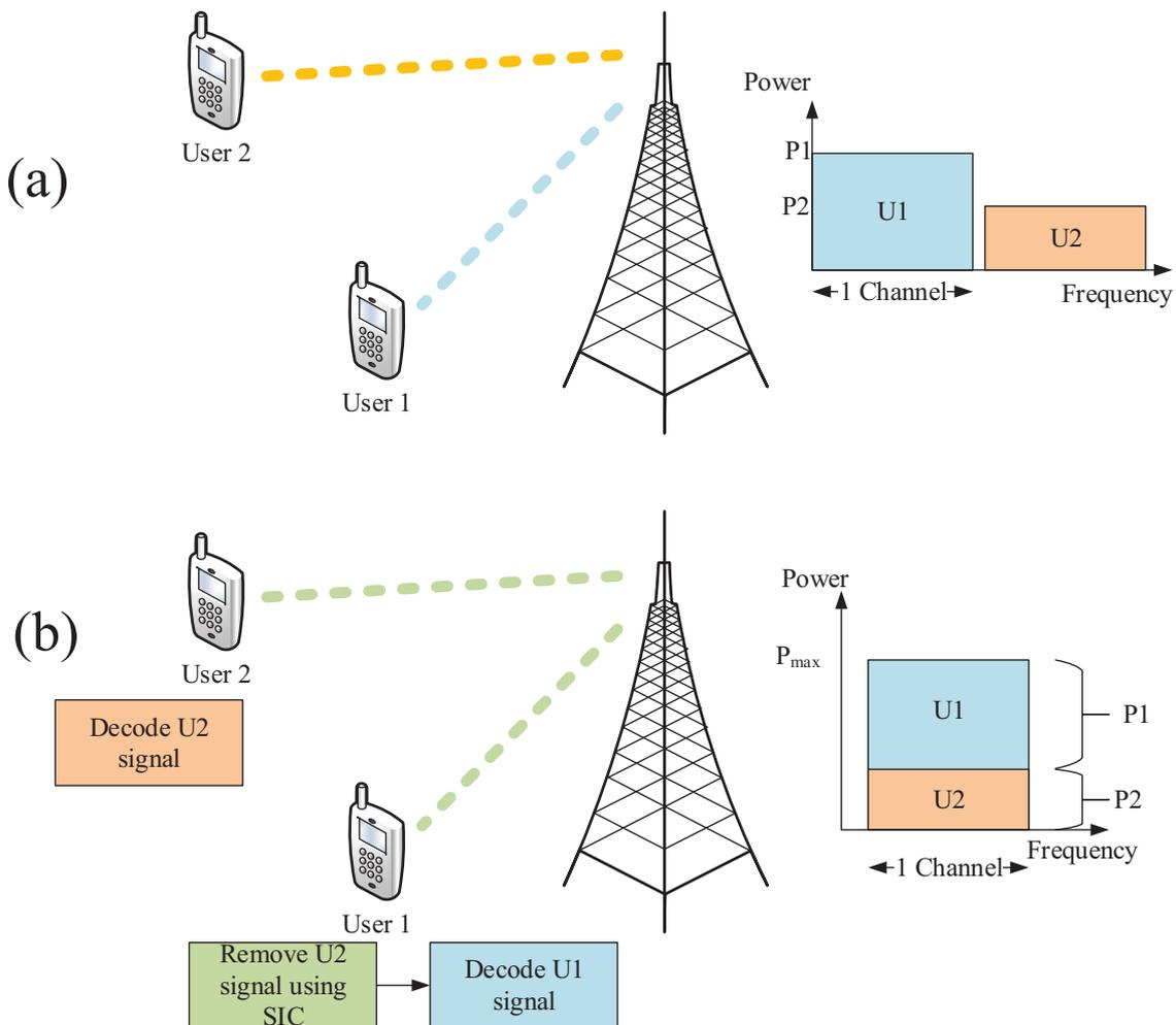
**Figure 1.** Conceptual comparison between (a) orthogonal multiple access (OMA) and (b) non-orthogonal multiple access (NOMA).
