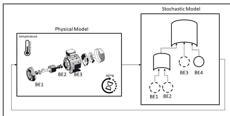
Figure 9. The SHyFTA model of an electric motor.
