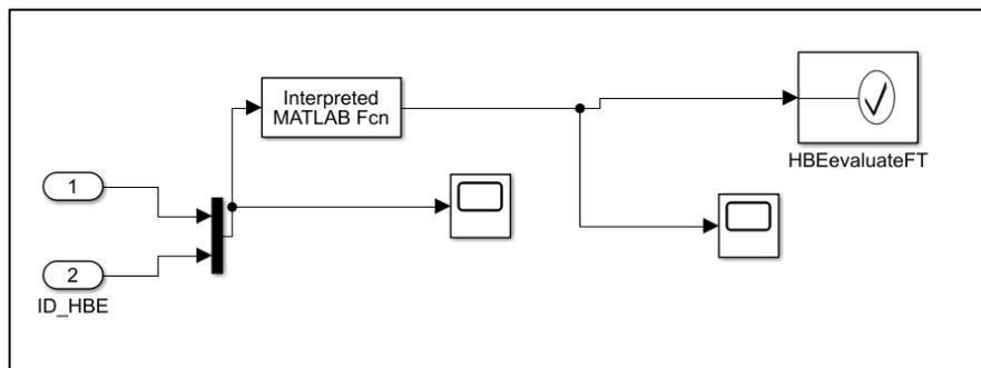
Figure 7. The Simulink implementation of the hybrid basic event HBE6.
