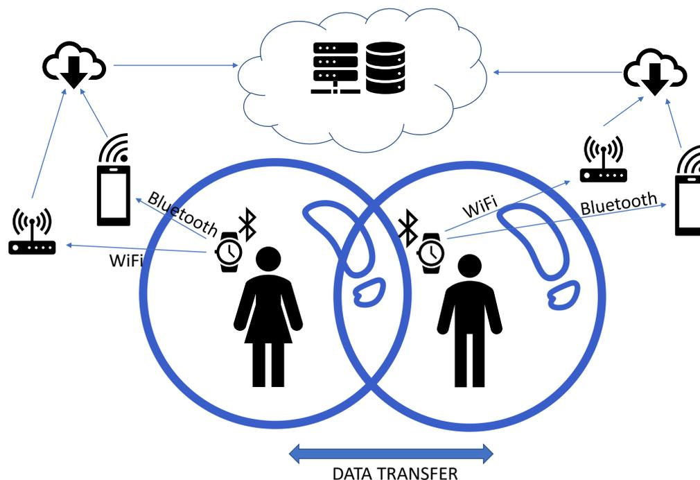
**Figure 1.** The BubbleBox system is composed of a device, i.e., a wristband to log unsafe contacts, an app, to pair devices and the identities of people wearing them, and a server infrastructure to store data and make it available of the authorized medical personnel.
