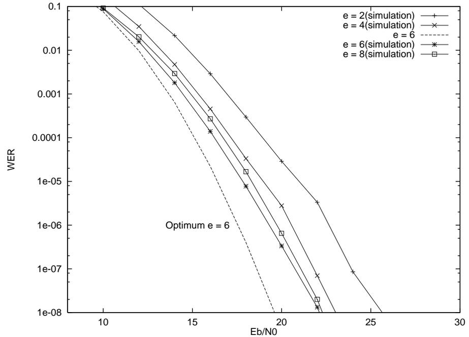
Figure 5. WER vs.  $E_b/N_0$  for truncation only with ordering.
