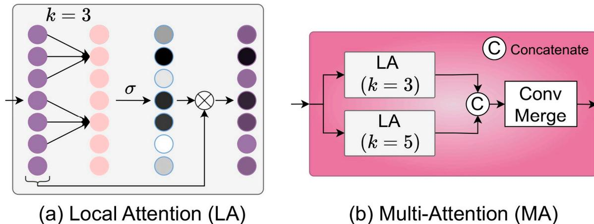
**Figure 4.** Schematic representation of proposed (a) local attention (LA) and (b) multi-attention (MA) modules.
