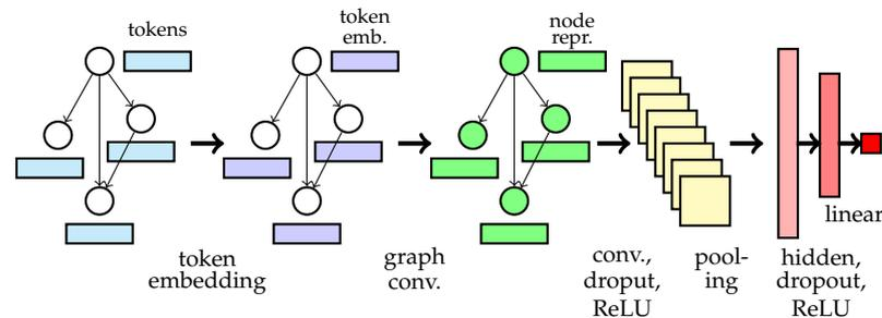
**Figure 4.** Architecture of models. In our 3-property encoding, the number of tokens of each node is 3. In code-based encoding, each node has the number of tokens of the node that has the most tokens.
