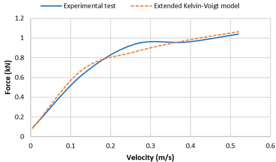
**Figure 6.** Force vs. velocity: Experimental tests and extended Kelvin–Voigt model.
