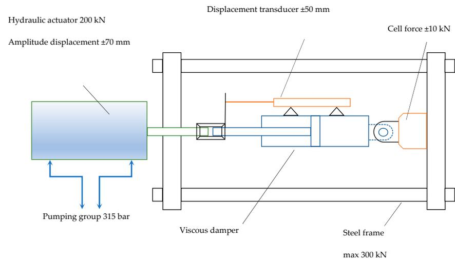
Figure 2. Experimental setup.
