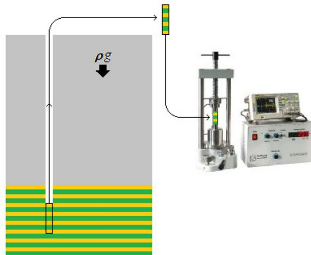
Figure 6. Extraction of a core sample from a stressed massif for investigation.
