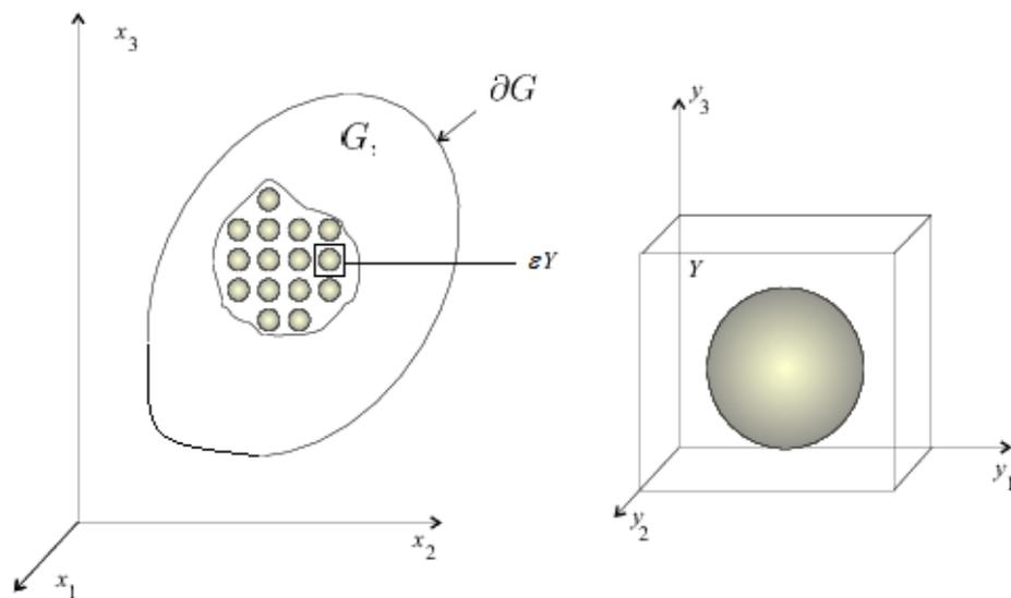
Figure 1. Body of periodic structure—left, and its periodicity cell—right.
