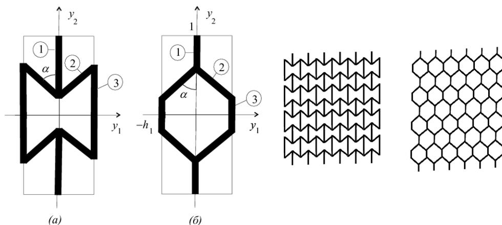
**Figure 4.** Honeycomb-like periodicity cells: (a) inverted honeycomb-like cell and (b) standard honeycomb cell and the corresponding composites.
