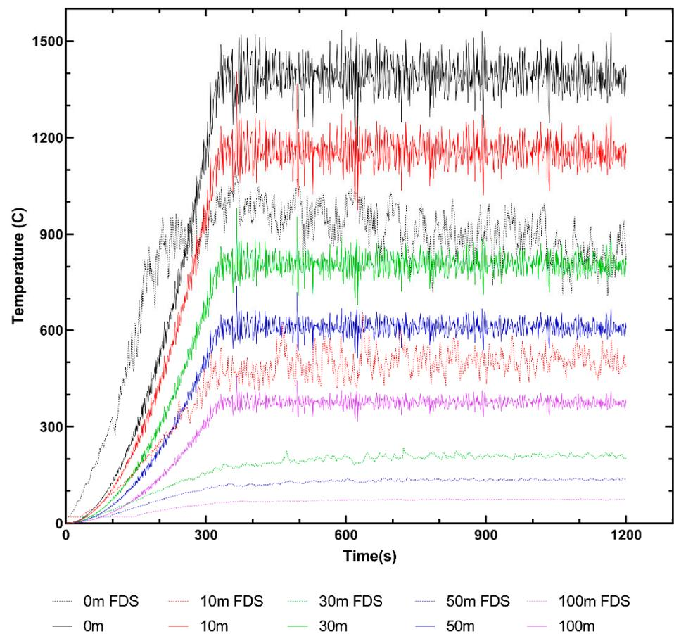
**Figure 2.** Comparison of the tunnel ceiling gas temperatures calculated with the empirical model with the values extracted by the numerical simulation at different distances above the fire source.
