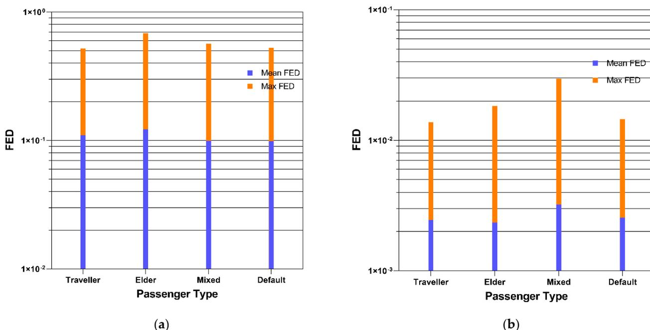
**Figure 6.** Mean and max FED index values for each passenger type for the (a) ventilated and (b) non-ventilated scenarios. The values never exceed the critical value of 1 but in the ventilated scenario the FED values are an order of magnitude higher than the non-ventilated one.
