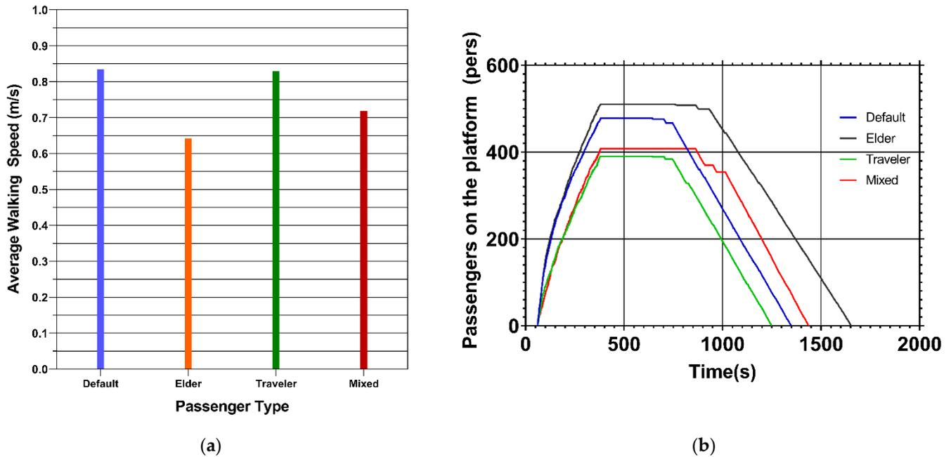
**Figure 5.** (a) Average passenger walking speed and (b) evacuation times for each passenger profile. As shown, the mixed population has lower average walking speed than the default and traveler group. As for the evacuation times, travelers may have the same speed as the default passengers, but their dimensions do not allow for a higher flow rate through the train doors. This limits the number of passengers that can evacuate to the platform in a given time.
