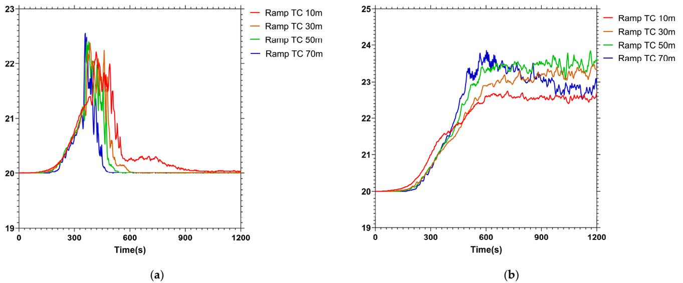
**Figure 4.** Upwind fire temperature distribution at  $y = 0.5$  m (symmetry plane of the walking platform) and 2 m height for (a) the ventilated scenario and (b) the non-ventilated scenario. The temperature does not exceed 24 degrees; thus, the evacuation can be carried out.
