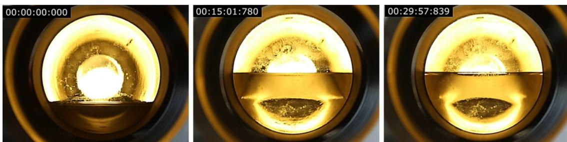
**Figure 5.** Kinetics of the change in the “2-propanol—CO<sub>2</sub>” system liquid phase volume without the addition of the alginate gel at a temperature of 312.68 K and a pressure of 7.98 MPa.
