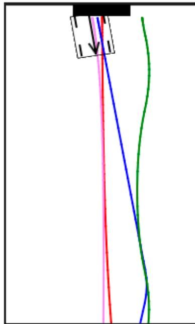
**Figure 1.** The trajectory of movement of a mobile object (Trajectories marked with different colors correspond to inference engine implementations that are based on different representations of fuzzy logic operations).
