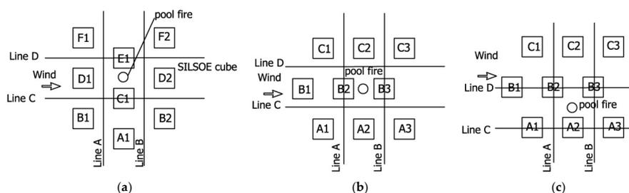
**Figure 1.** Model city buildings arrangement (marked squares), diesel pool fire location (circle) and wind direction (arrow) for (a) Case 1 where the Silsoe cube is also indicated; (b) Case 2; and (c) Case 3.
