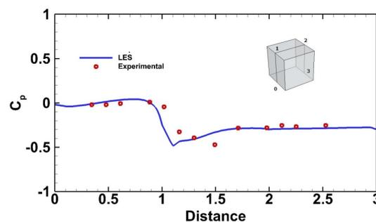
**Figure 2.** Pressure coefficient around the Silsoe Cube situated in the building array of Case 1, with “-” as the present results and with “o” as the measurements from the King, Gough [45] experiments.
