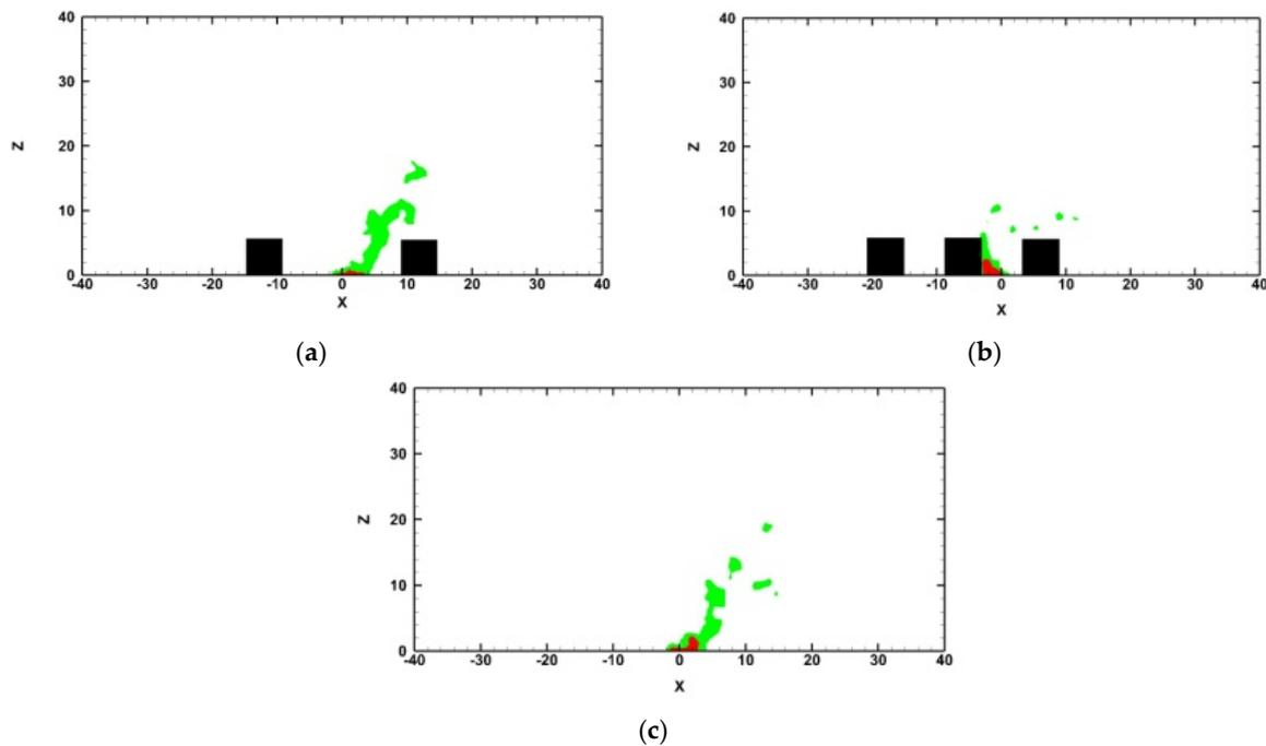
**Figure 11.** The LC1 zone and the IDLH zone at the fire's symmetry for (a) Case 1; (b) Case 2; (c) Case 3 after 200 s of the fire incidence at the.
