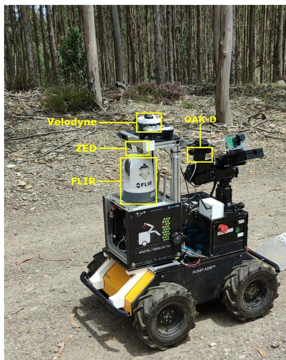
**Figure 3.** Lateral view of the ground mobile robotic platform AgRob V16 with the sensors annotated.
