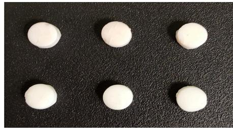
**Figure 1.** Circular-shaped study specimens with 0%, 0.5% and 1.0% wt.% GF incorporated in GIC (from left to right). The upper row denotes specimens prepared with KCR, while the lower row links to specimens prepared with MC.
