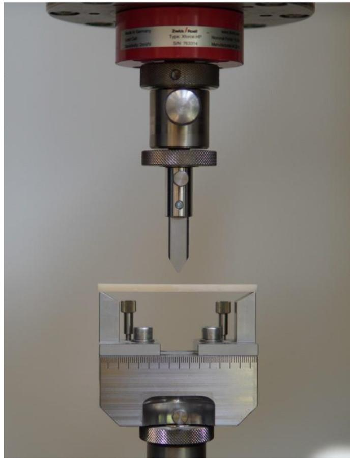
**Figure 4.** Three-point flexure test setup.
