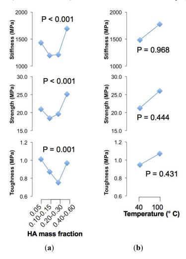
**Figure 1.** Main effect plots. (**a**) Plot of the mean value of the respective mechanical properties (averaged over the values of the respective specimens for the different crystallization temperatures) *versus* hydroxyapatite (HA) concentration; (**b**) Plot of the mean value of the respective mechanical properties (averaged over the values of the respective specimens for the different HA concentrations) *versus* crystallization temperature.
