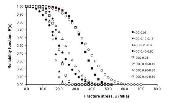
**Figure 3.** Plot of reliability function,  $R(\sigma)$ , *versus* fracture stress in the fibre,  $\sigma$ , at varying hydroxyapatite (HA) concentrations and crystallization temperatures. Note:  $R(\sigma) = \exp(-(\sigma/\sigma_0)^{\beta})$ , where  $\sigma_0$  and  $\beta$  are the characteristic strength and the Weibull modulus, respectively.
