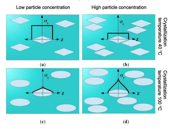
**Figure 4.** Schematic of HA-nanoparticle-reinforced chitosan composite fibre. (**a**,**c**) and (**b**,**d**) depict HA in the chitosan matrix at low and high concentrations, respectively; (**a**,**b**) and (**c**,**d**) depict HA particles corresponding to crystallization temperature at 40 and 100 °C, respectively. Overlaying one of the particles in each panel is a sketch of the graph of axial stress ( $\sigma_z$ ) in the particle versus distance (*z*) along the particle axis.
