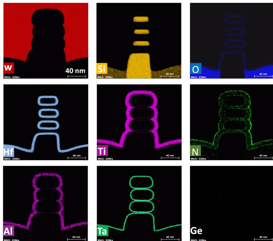
**Figure 3.** The EDS images of NSFETs in this work. The top figures illustrate W, Si, and O elements. The middle figures illustrate Hf, Ti, and N elements. The bottom figures illustrate Al, Ta, and Ge elements. Ge has been removed completely.
