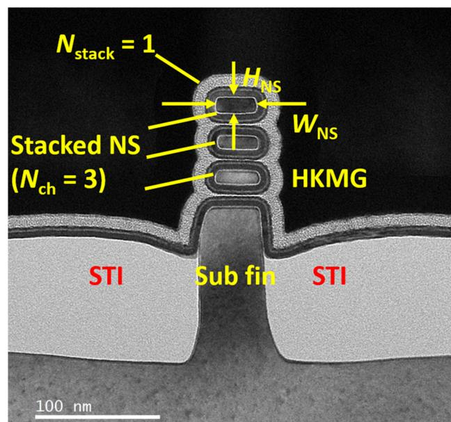
**Figure 2.** The TEM image of GAA NSFETs in this work. The nanosheets are separated from each other.
