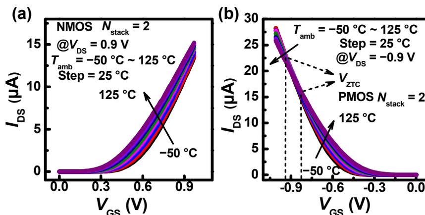
**Figure 4.** Experimental temperature dependence of transfer characteristics at  $L_G = 500$  nm,  $N_{stack} = 2$ , (a)  $V_{DS} = 0.9$  V for NMOS and (b)  $V_{DS} = -0.9$  V for PMOS. It shows two  $V_{ZTC}$  under  $T_{amb} = -50\sim 25$  °C range and  $T_{amb} = 25\sim 125$  °C range.
