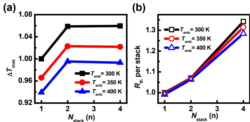
**Figure 12.** When  $V_{\text{GS}} = V_{\text{DS}} = 0.7\text{ V}$ , (a)  $\Delta T_{\max}$  and (b)  $R_{\text{th}}$  variations relative to the devices with  $N_{\text{stack}} = 1$  under  $T_{\text{amb}} = 300\text{ K}$ .
