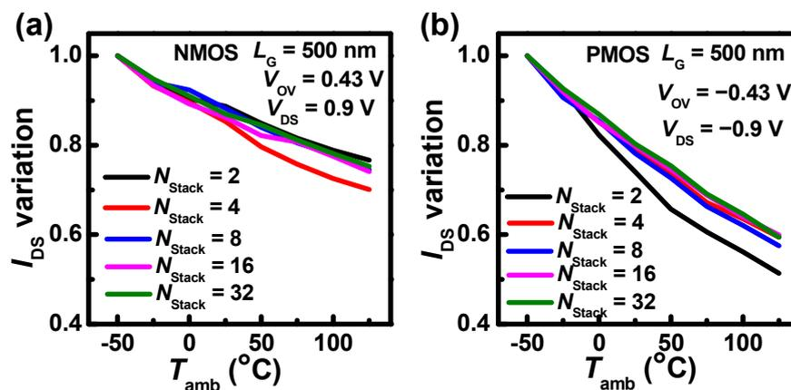
**Figure 5.** (a)  $I_{DS}$  variations of NMOS with different  $N_{stack}$ s under the impact of  $T_{amb}$  relative to the  $I_{DS}$  at  $T_{amb} = -50$  °C, (b)  $I_{DS}$  variations of PMOS with different  $N_{stack}$ s under the impact of  $T_{amb}$  relative to the  $I_{DS}$  at  $T_{amb} = -50$  °C.
