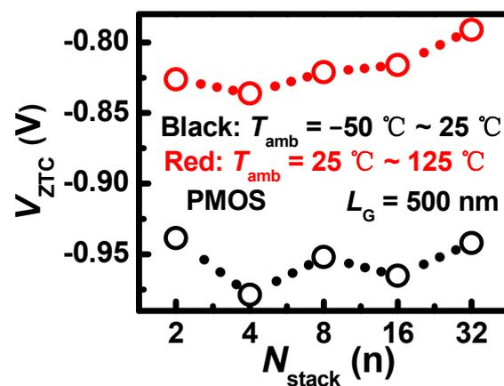
**Figure 8.**  $L_G = 500\text{ nm}$ , the  $V_{ZTC}$  of PMOS with different  $N_{stack}$  under  $T_{amb} = -50\text{--}25\text{ }^\circ\text{C}$  range and  $T_{amb} = 25\text{--}125\text{ }^\circ\text{C}$  range.
