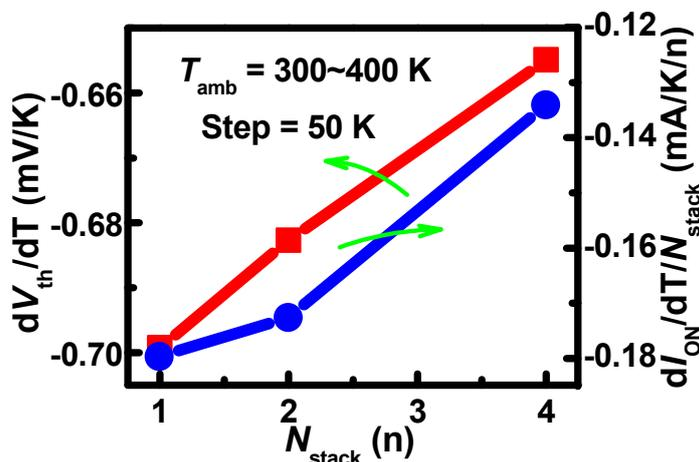
Figure 11. The temperature coefficients of  $V_{th}$  and the temperature coefficients of  $I_{DS}$  per stack with different  $N_{stack}$ s.
