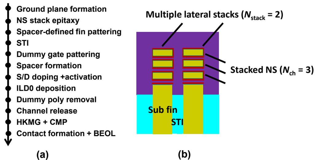
**Figure 1.** (a) Process flow of GAA NSFETs adopting the gate last process. (b) Schematic of the NSFET with multiple lateral stacks along the nanosheet width direction.
