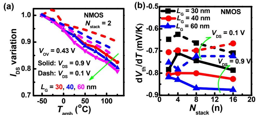
**Figure 9.** (a)  $I_{DS}$  variations with different gate lengths under the impact of  $T_{amb}$  relative to the  $I_{DS}$  at  $T_{amb} = -50$  °C. (b) The temperature coefficients of  $V_{th}$  with different gate lengths when the  $N_{stack}$  increases.
