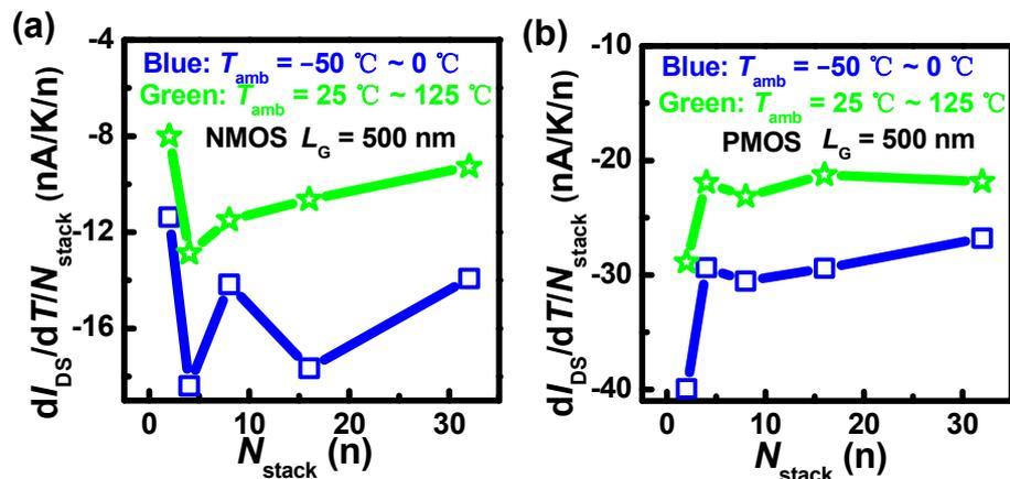
Figure 6.  $L_G = 500\text{ nm}$ , (a)  $V_{DS} = 0.9\text{ V}$ ,  $V_{ov} = 0.59\text{ V}$ , the temperature coefficients of  $I_{DS}$  per stack in NMOS, (b)  $V_{DS} = -0.9\text{ V}$ ,  $V_{ov} = -0.59\text{ V}$ , the temperature coefficients of  $I_{DS}$  per stack in PMOS under different  $T_{amb}$  ranges.
