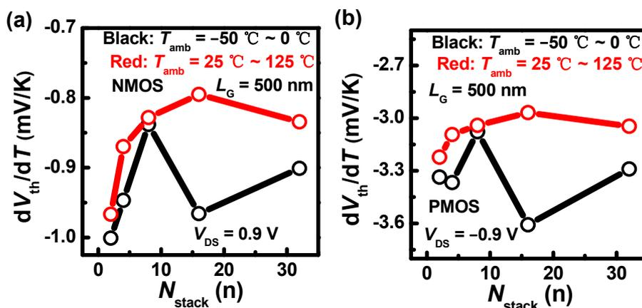
Figure 7.  $L_G = 500\text{ nm}$ , the temperature coefficients of  $V_{th}$  ( $\eta$ ) with different  $N_{stack}$ 's in (a) NMOS and (b) PMOS under different  $T_{amb}$  ranges.
