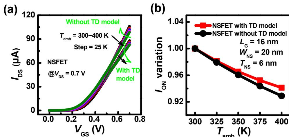
Figure 10. (a) The transfer characteristics of NSFET ( $N_{stack} = 1$ ) with/without the SHE as the  $T_{amb}$  increases from 300 K to 400 K, (b)  $I_{DS}$  variations relative to the  $I_{DS}$  at  $T_{amb} = 300$  K with/without the SHE when  $V_{GS} = V_{DS} = 0.7$  V.
