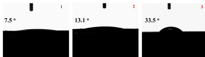
**Figure 2.** Images of water contact angles of (1) MC, (2) MCC, and (3) NC samples.
