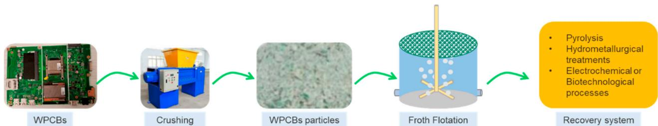
**Figure 3.** Schematic of the e-waste froth flotation process.
