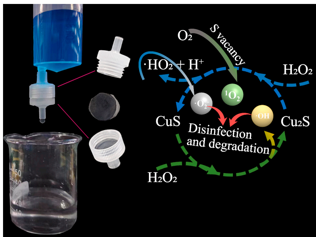
Figure 9. Design of novel device for wastewater treatment using CSCM-SRB with Fenton-like mechanism.
