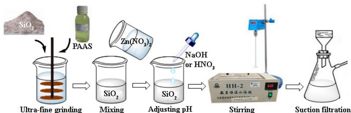
Figure 2. Preparation of composite particles of ZnO–SiO<sub>2</sub> precursor.
