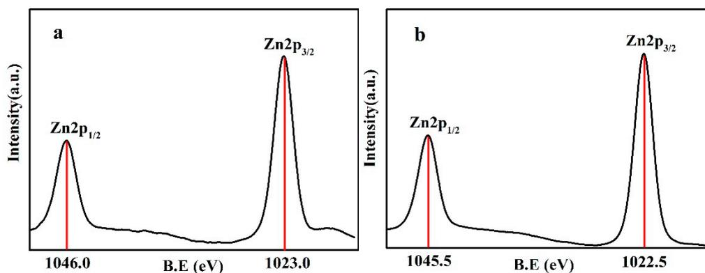
Figure 6. XPS of (a) ZnO–SiO<sub>2</sub>-pH5.0; (b) ZnO–SiO<sub>2</sub>-pH7.0.
