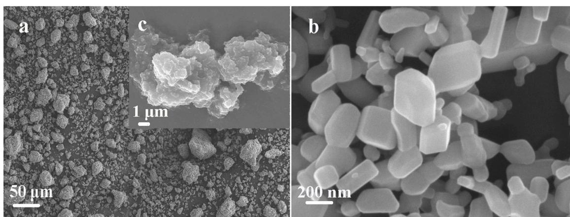
Figure 1. Micrographs of (a,c) amorphous  $\text{SiO}_2$  and (b) pure ZnO.
