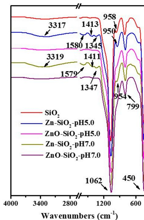
Figure 7. FTIR spectra of amorphous SiO<sub>2</sub>, Zn–SiO<sub>2</sub>-pH5.0, ZnO–SiO<sub>2</sub>-pH5.0, Zn–SiO<sub>2</sub>-pH7.0, and ZnO–SiO<sub>2</sub>-pH7.0.
