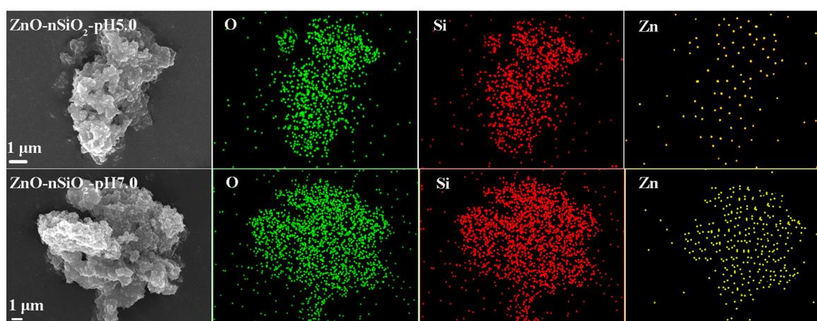
**Figure 4.** SEM images of ZnO–SiO<sub>2</sub> and corresponding mapping results.
