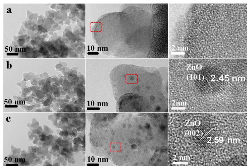
**Figure 5.** TEM maps of (a) amorphous SiO<sub>2</sub>; (b) ZnO-SiO<sub>2</sub>-pH5.0; (c) ZnO-SiO<sub>2</sub>-pH7.0 at different scales.
