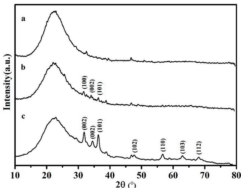
Figure 3. XRD of (a) amorphous SiO<sub>2</sub>; (b) ZnO–SiO<sub>2</sub>-pH5.0; and (c) ZnO–SiO<sub>2</sub>-pH7.0.
