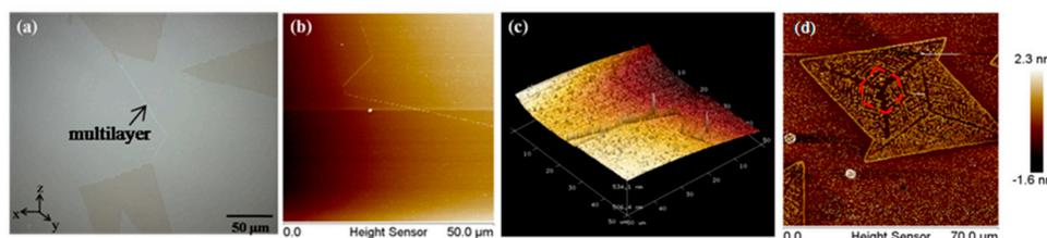
**Figure 4.** (a) optical image on the grain boundary; (b) 2D image of the grain boundary by atomic force microscope (AFM); (c) 3D image of the grain boundary by AFM; (d) outline of the film by AFM.
