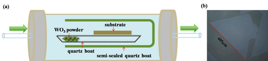
**Figure 2.** (a) Semi-sealed equipment schematic diagram; (b) optical microscope of  $405\ \mu\text{m}$  monolayer  $\text{WS}_2$  film.
