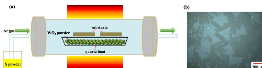
**Figure 1.** (a) Schematic diagram of CVD growth system; (b) optical image of  $\text{WS}_2$ .
