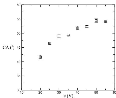
**Figure 2.** Contact angle versus AAO processing voltage.
