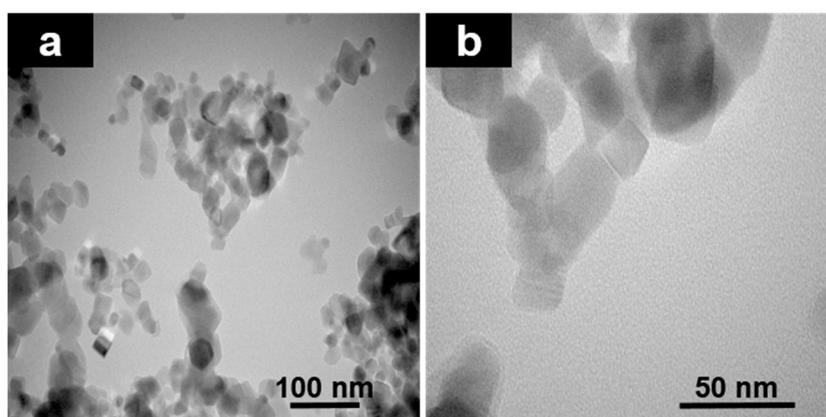
**Fig. 4SI.** SEM images of TiO<sub>2</sub> NPs at different magnifications: (a) 60 k $\times$  and (b) 200 k $\times$ .
