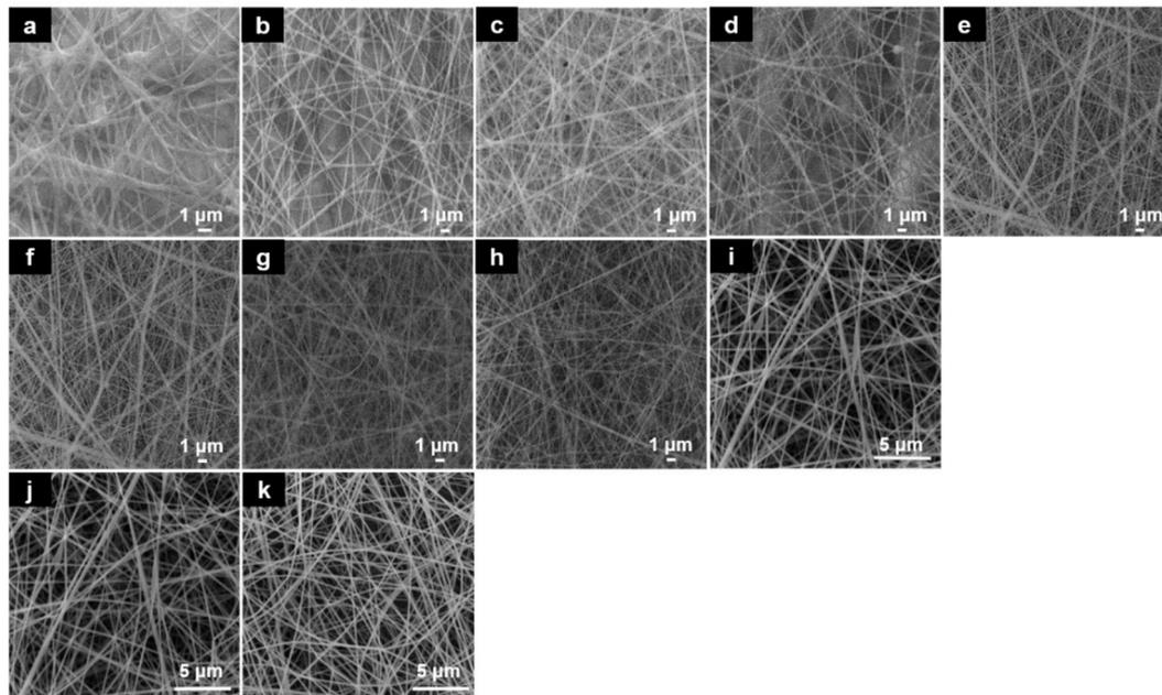
**Fig. 2SI.** SEM images of PVN according to conditions expressed in Table 1SI: (a–e) variation of needle diameter; (f–i) variation of flow rate; and (j–k) variation of the distance. All samples presented magnification 25000x.
