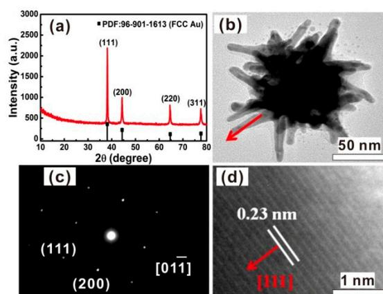
**Figure 3.** (a) XRD pattern of the chestnut-like Au nanocrystals. The line spectrum is the standard pattern of Au powders. (b) TEM image of an individual chestnut-like Au nanocrystal. (c) Selected area electron diffraction (SAED) pattern of the particle in (b). (d) HRTEM image of the nanoneedle marked with an arrow in (b). The arrows in (b,d) are parallel.
