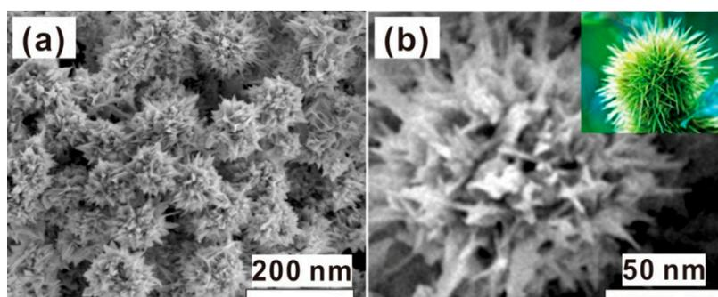
**Figure 2.** The field emission scanning electron microscope (FESEM) images of the as-prepared products. (a) The image with low magnification. (b) The magnified image of the single particle in (a). The inset is the photo of one chestnut for reference.
