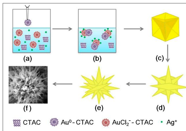
**Figure 7.** Schematic illustration for the formation of the chestnut-like Au nanocrystals. (a) The seeds were dropped into the growth solution. (b)  $\text{AuCl}_2^-$  complex was reduced onto the surface of  $\text{Au}^0$  using electrons from ascorbic acid in the growth solution. (c) Formation of concave nanocubes during the initial growth period. (d) The radial growth of [111]-oriented nanoneedles. (e) The branched growth on the formed nanoneedles. (f) The chestnut-like Au nanocrystal.
