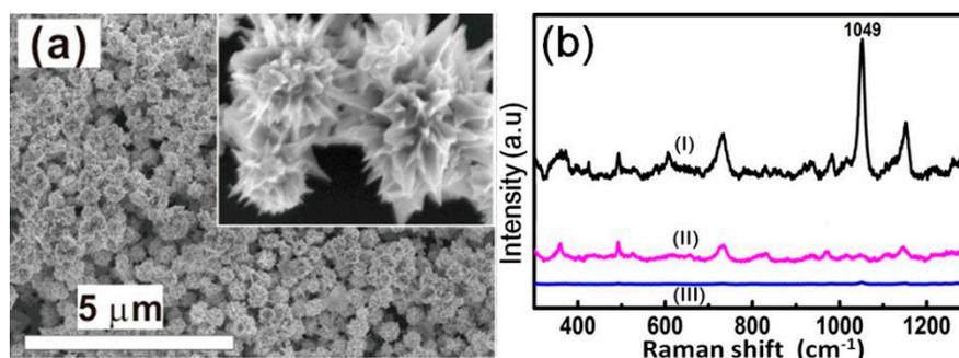
**Figure 8.** (a) The FESEM image of the as-prepared chestnut-like Au nanocrystals-built film (~500 nm in thickness) on a silicon substrate. The inset is the local magnified image. (b) The Raman spectra of the chestnut-like Au nanocrystals-built film after argon plasma bombardment for different times. Curves (I, II, III): after bombardment for 0 min, 5 min, and 10 min, respectively.
