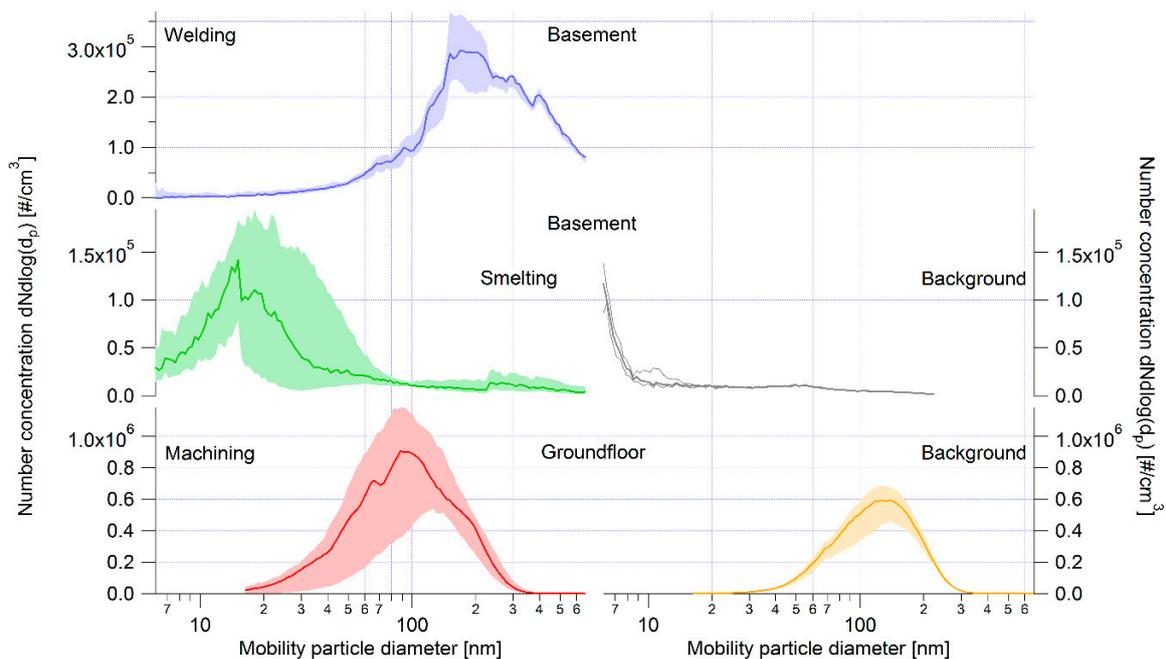
**Figure S1.** Particle number size distributions during welding, smelting, and machining (grinding and milling), and corresponding backgrounds measured by SMPS; solid line represents median for the measurement period and the corresponding shaded area shows interquartile span.
