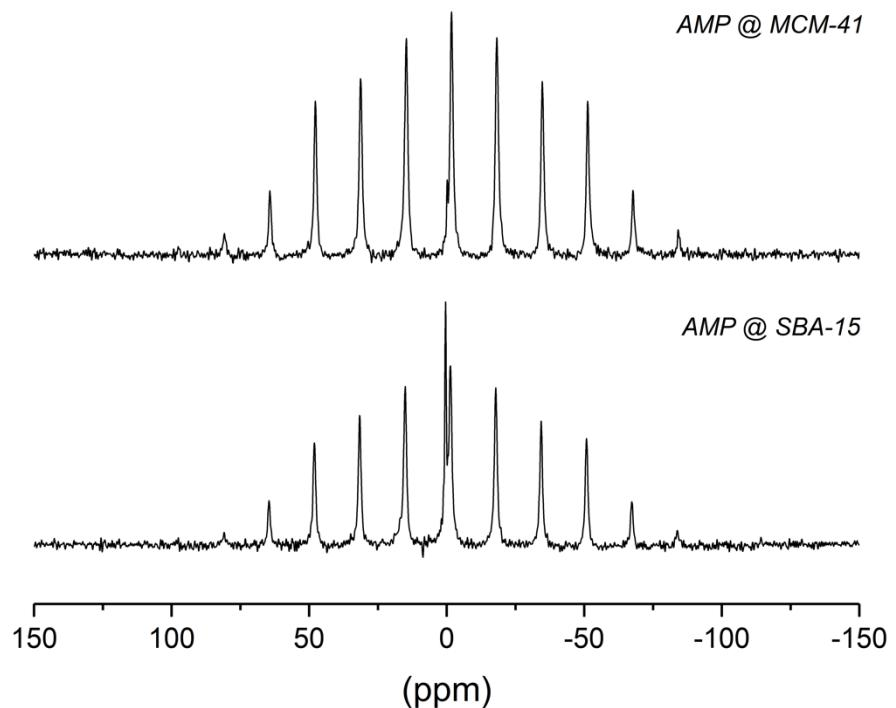
**Figure S5.**  $^{31}\text{P}$  MAS NMR spectra of AMP (2)-loaded silica (MCM-41 and SBA-15).
