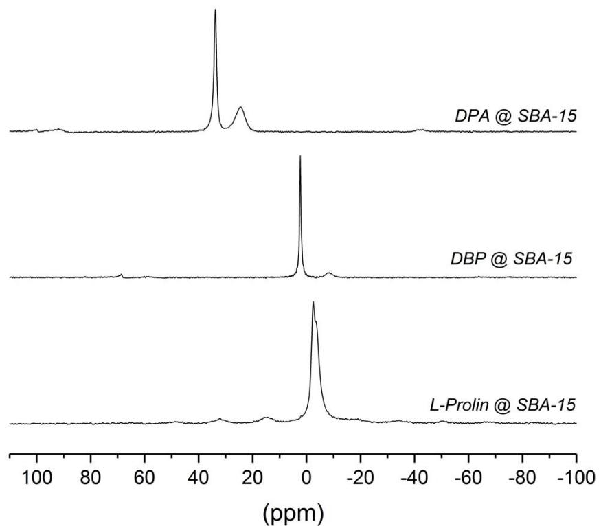
**Figure S6.**  $^{31}\text{P}$  MAS NMR spectra of SBA-15-functionalized with DPA (3), DBP (4) and (4R)-4-phosphonoxy
