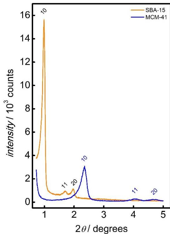
**Figure S2.** Low angle X-ray diffraction of SBA-15 and MCM-41.
