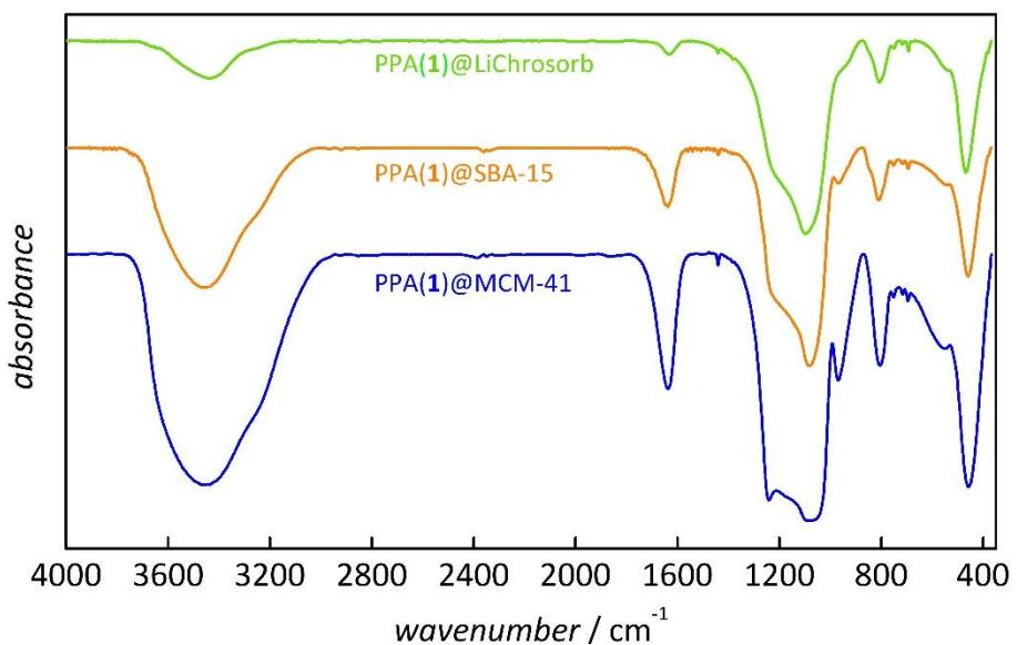
**Figure S3.** FTIR spectra of PPA(1)-functionalized silica (LiChrosorb, SBA-15, MCM-41).
