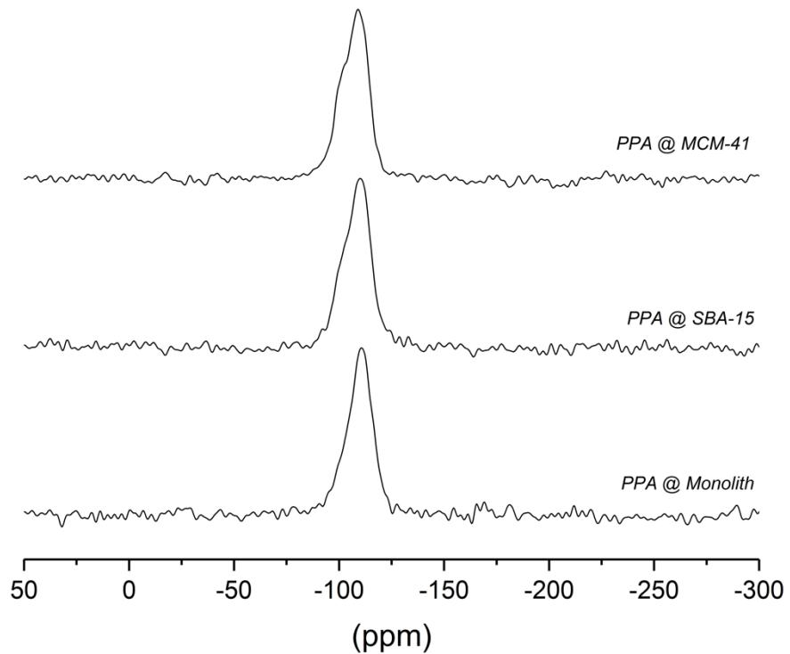
**Figure S4.** <sup>29</sup>Si MAS NMR spectra of PPA (1)-functionalized silica (MCM-41, SBA-15 and monolith).
