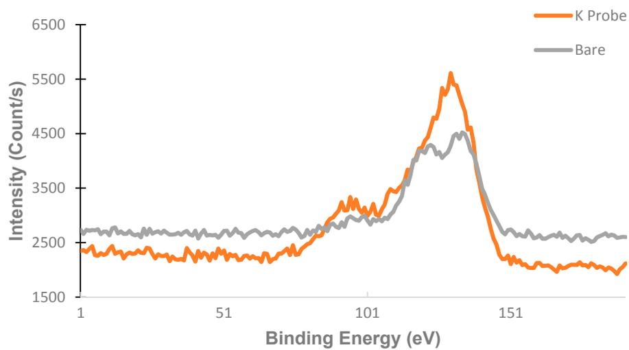
**Figure S-4:** X-Ray Photoelectron Spectroscopy (XPS) narrow scans for gold microelectrode for carbon. Bare cleaned gold was compared to gold coated with a mixed monolayer of K<sup>+</sup> probe and MEG-SH in a 1:10 ratio.
