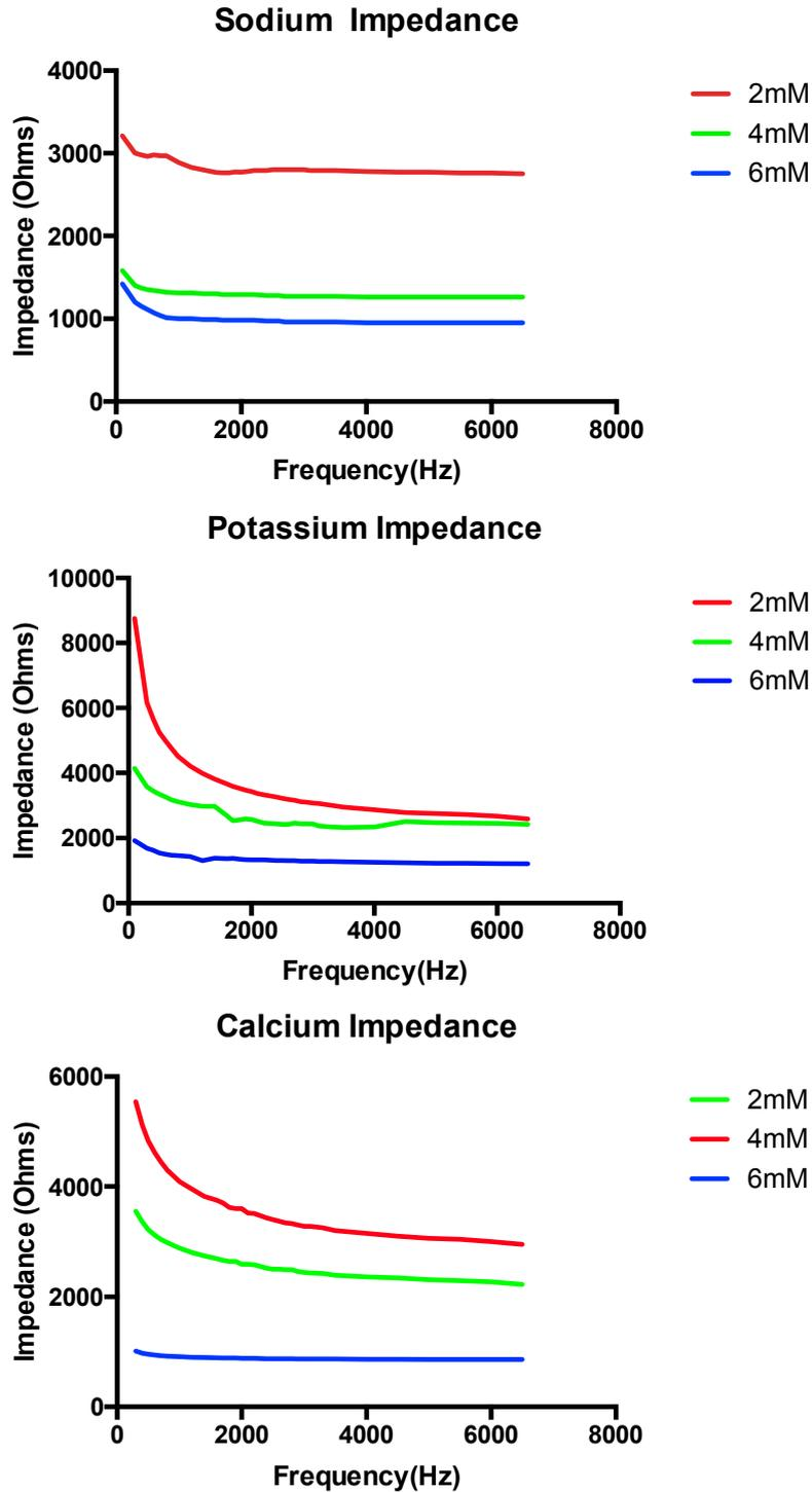
**Figure S-3:** Impedance measurements for: sodium(top), potassium(middle), and calcium(bottom) in simulated cerebrospinal fluid (CSF). Each solution contained: NaCl 120mM, 10 mM glucose 10mM, NaHCO<sub>3</sub> 22mM, NaH<sub>2</sub>PO<sub>4</sub>·H<sub>2</sub>O, MgSO<sub>4</sub> mM and CaCl<sub>2</sub> 2.6mM. Any compounds containing the cation of interest in the simulated CSF were replaced with a similar cation.
