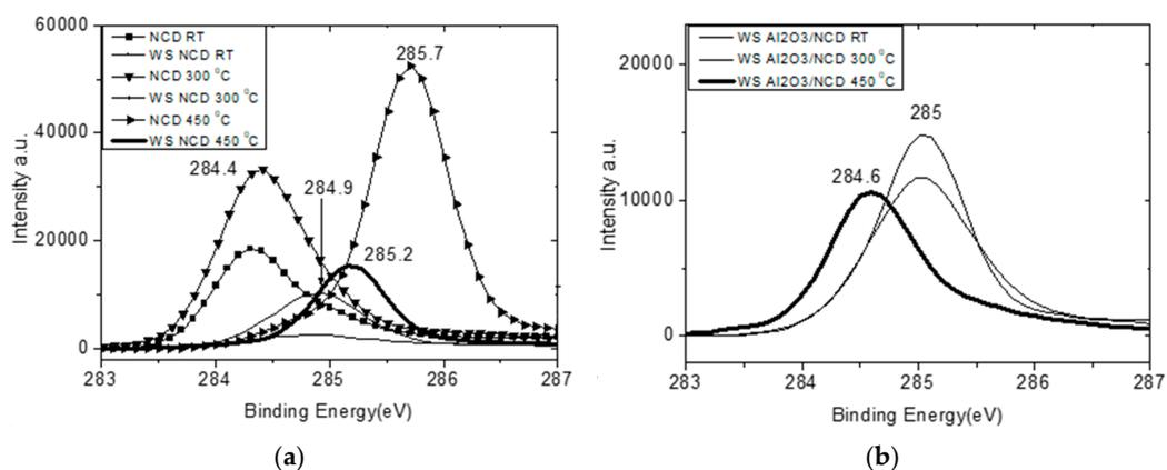
Figure 12. XPS spectra of the C 1s peak taken on the (a) NCD and (b) Al<sub>2</sub>O<sub>3</sub>/NCD films.
