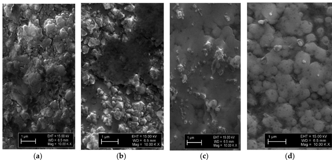
**Figure 5.** SEM images taken on the wear scar after the test at RT on the Al<sub>2</sub>O<sub>3</sub>/NCD film. The images were taken from (a) the center of the wear scar (b,c) were taken in the middle of the wear scar to (d) the border of the wear scar images.
