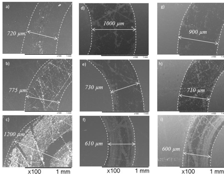
**Figure 7.** SEM images of the wear scars after sliding tests on the NCD film at (a) RT, (b) 300 °C and (c) 450 °C;  $\text{Al}_2\text{O}_3/\text{NCD}$  film at (d) RT, (e) 300 °C and (f) 450 °C; and  $\text{A-Al}_2\text{O}_3/\text{NCD}$  film at (g) RT, (h) 300 °C and (i) 450 °C.
