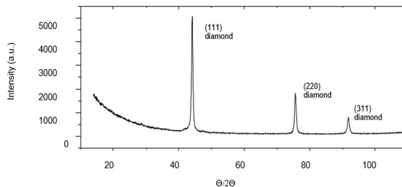
Figure 2. XRD pattern measured on the as-deposited  $\text{Al}_2\text{O}_3/\text{NCD}$  film.
