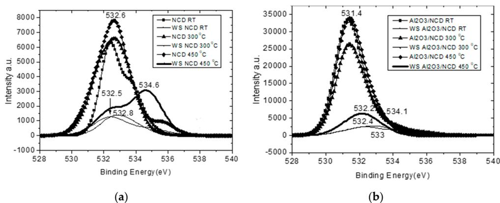
**Figure 11.** XPS spectra of the O 1s peak (WS-wear scar) taken on the (a) NCD and (b) Al<sub>2</sub>O<sub>3</sub>/NCD films.
