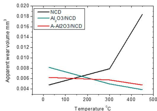
**Figure 9.** Apparent wear volumes of the wear scars measured on the NCD,  $\text{Al}_2\text{O}_3/\text{NCD}$  and A- $\text{Al}_2\text{O}_3/\text{NCD}$  films.
