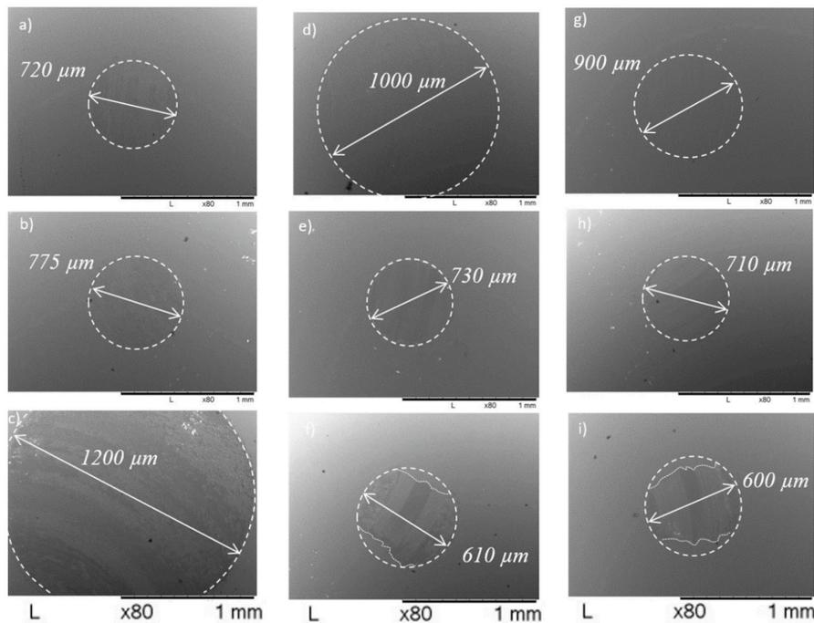
**Figure 8.** SEM images of the worn surface on the balls after sliding tests against the NCD film at (a) RT, (b) 300 °C and (d) 450 °C;  $\text{Al}_2\text{O}_3/\text{NCD}$  film at (d) RT, (e) 300 °C and (f) 450 °C; and A- $\text{Al}_2\text{O}_3/\text{NCD}$  film at (g) RT, (h) 300 °C and (i) 450 °C.
