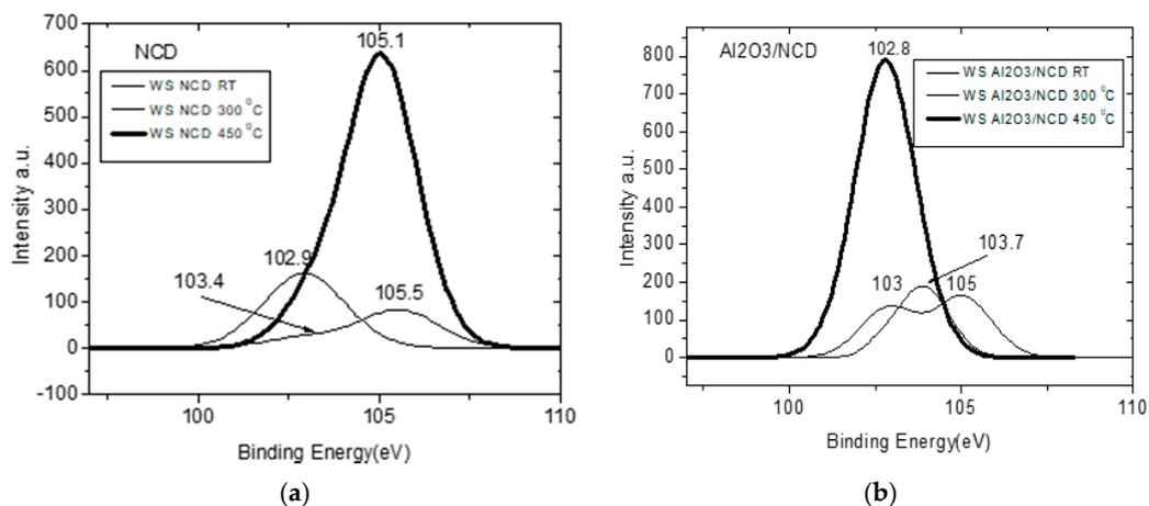
**Figure 14.** XPS spectra of the Si 2p peak taken on the (a) NCD and (b) Al<sub>2</sub>O<sub>3</sub>/NCD films.
