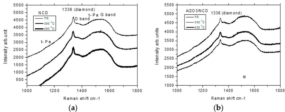
**Figure 10.** Raman spectra taken on the (a) NCD and (b) Al<sub>2</sub>O<sub>3</sub>/NCD films.
