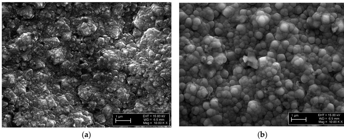
Figure 1. (a) SEM images of the NCD and (b)  $\text{Al}_2\text{O}_3/\text{NCD}$  films.
