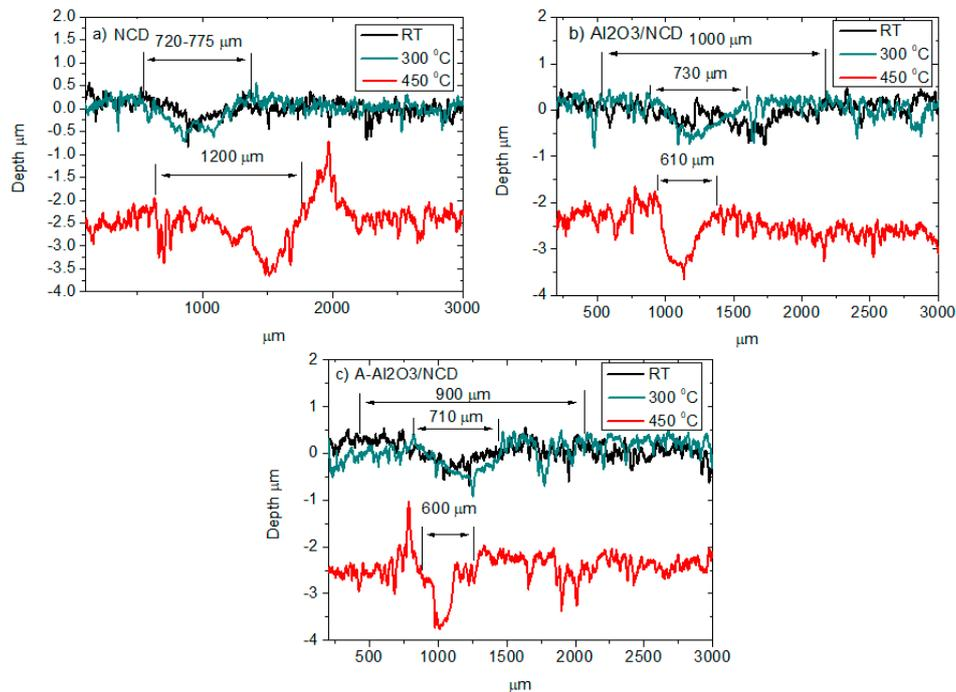
**Figure 6.** Line scans across the wear scars taken on the (a) NCD, (b)  $\text{Al}_2\text{O}_3/\text{NCD}$  and (c)  $\text{A-Al}_2\text{O}_3/\text{NCD}$  films.
