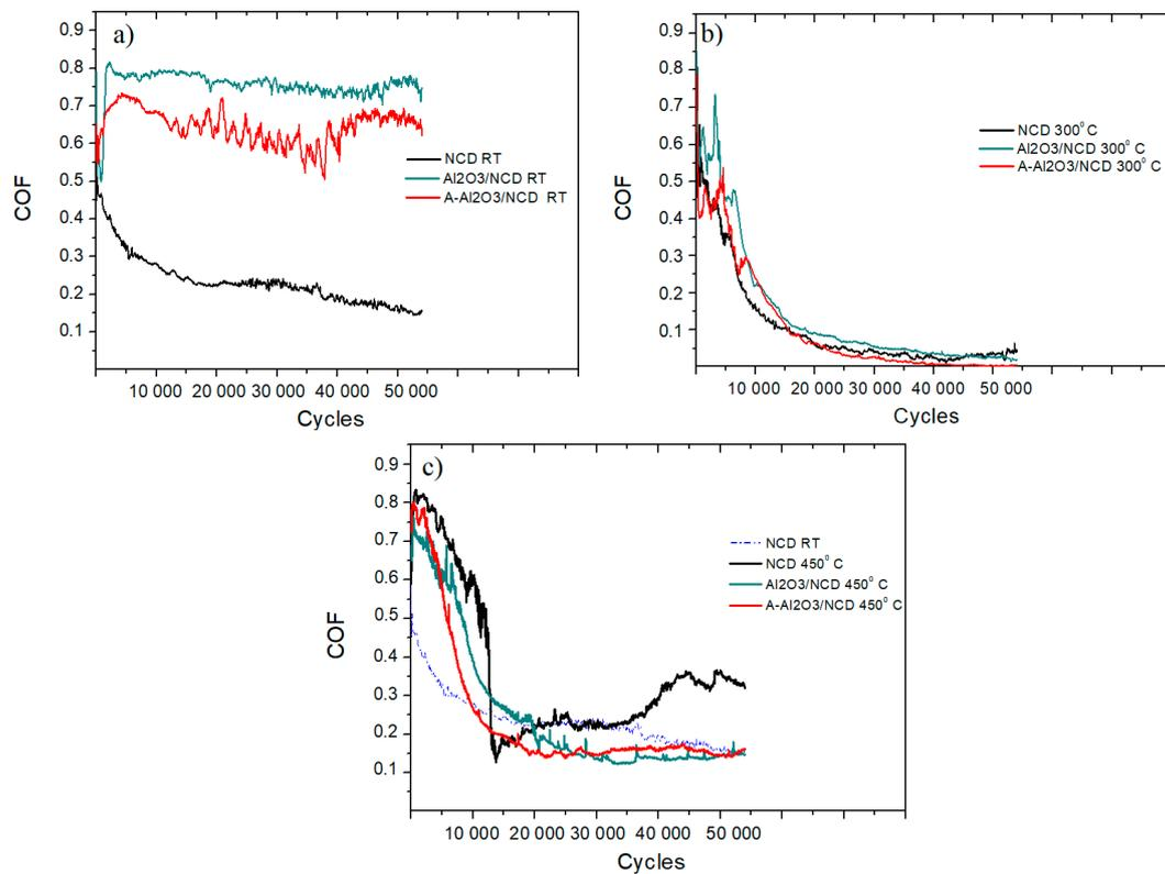
**Figure 3.** COF vs number of cycle curves taken on the NCD, Al<sub>2</sub>O<sub>3</sub>/NCD and A-Al<sub>2</sub>O<sub>3</sub>/NCD films at (a) RT, (b) 300 °C and (c) 450 °C.
