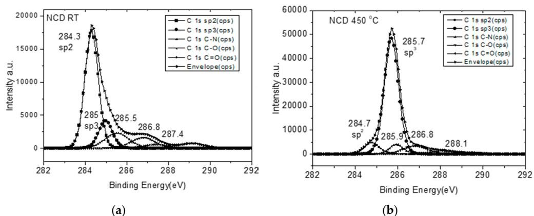
Figure 13. XPS spectra of the C 1s peak taken on the NCD film native surface at (a) RT and after the heating at (b) 450 °C.
