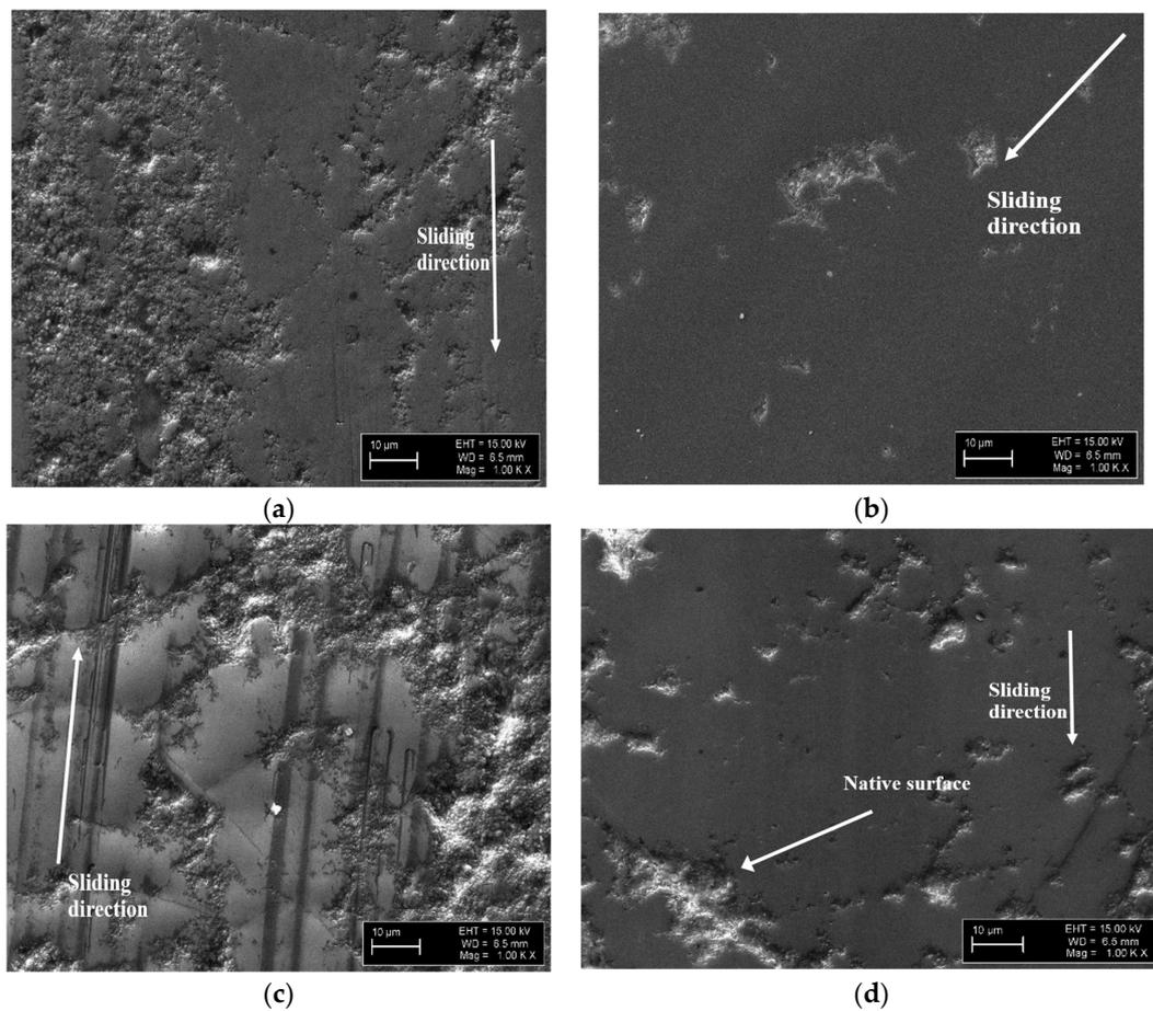
**Figure 4.** Surface morphology of the wear scars after the tests on the NCD film at (a) 300 °C and (b) 450 °C, and on the Al<sub>2</sub>O<sub>3</sub>/NCD film at (c) 300 °C and (d) 450 °C.
