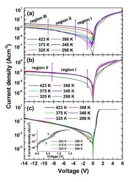
**Figure 2.** Semilogarithmic current–voltage (I–V) data obtained at different temperatures for samples (**a**) A, (**b**) B, and (**c**) C. The inset in (**c**) shows the I–V curves for narrow forward bias range obtained from sample C.
