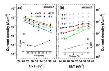
**Figure 7.** Reverse leakage current density vs. temperature at different reverse biases for samples (**a**) A and (**b**) C. The insets in (**a**) and (**b**) show the obtained activation energies for samples A and C, respectively.
