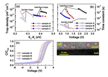
**Figure 9.** (a) Trap density vs. energy level, (b) time constant vs. voltage, (c) *C*–*V* hysteresis plots obtained at 100 kHz, and (d) cross-sectional scanning transmission electron microscopy (STEM) image for sample B.
