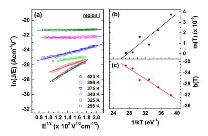
**Figure 4.** (a) Ln(J/E) vs.  $E^{1/2/}$  plots by the Poole–Frenkel (PF) emission model, together with the linear fitting to the experimental data for sample A. (**b**,**c**) The calculated *m* and *b* values, respectively.
