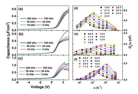
**Figure 8.** Capacitance–voltage (*C*–*V*) data at different frequencies for samples (**a**) A, (**b**) B, and (**c**) C, and frequency-dependent parallel conductance–voltage ( $G_p/\omega$ –*V*) curves for samples (**d**) A, (**e**) B, and (**f**) C.
