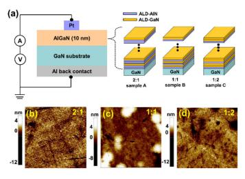
**Figure 1.** (a) Schematic layer structures of AlGaN/GaN devices and prepared AlGaN layers with different pulse ratios. (**b**–**d**) The atomic force microscopy (AFM) surface images scanned over  $2 \mu m \times 2 \mu m$  areas.
