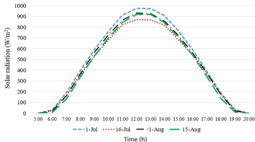
**Figure 9.** Hourly solar radiation in W/m<sup>2</sup> of different days of the site under study (during 2019).
