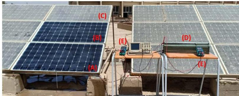
**Figure 6.** Picture of experimental set-up during measuring work. (A) Self-cleaning panel coated with  $\text{SiO}_2$  hydrophobic nanomaterial, (B) uncoated panel—manual cleaning, (C) dusty panel, over all the time of the experiment (reference), (D) load (variable resistance) and (E) measuring devices.
