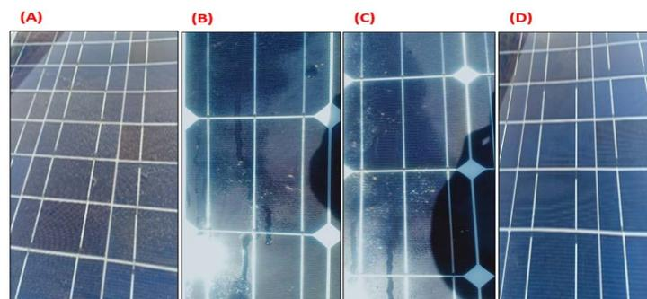
**Figure 7.** Process of surface self-cleaning with nano-coated material; starting from (A) dirty panel throughout (B) partially cleaned panel, then (C) almost cleaned panel, and finally (D) totally cleaned panel.
