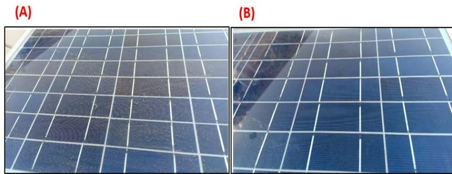
**Figure 12.** Anti-static effect of the solar PV panels. (A) non-coated panel (reference panel) (B) hydrophobic nano-coating SiO<sub>2</sub> material on the PV panel.
