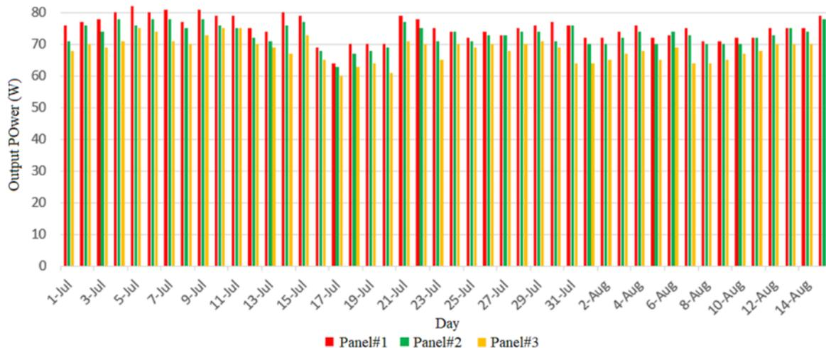
**Figure 11.** The average power generated by the three panels (during 2019); panel 1:  $\text{SiO}_2$  nano-coated panel; panel 2: manual cleaning panel without a coating of any material; panel 3: dusty panel.
