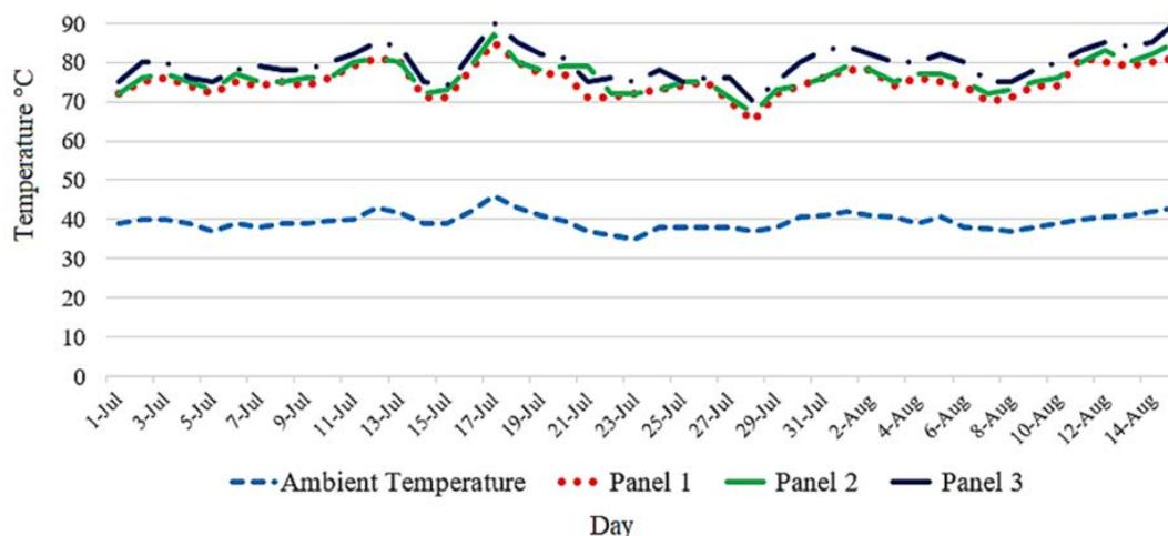
**Figure 14.** Average daily temperature; ambient and the three panels' temperatures at the maximum solar radiation per day.
