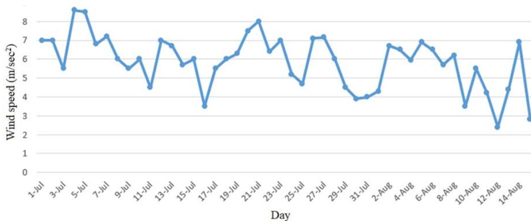
**Figure 13.** Measured wind speed at the site under study (Assiut University, Egypt) at the maximum solar radiation per day.
