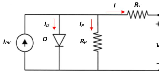
Figure 5. Equivalent circuit of the single diode model (SDM).
