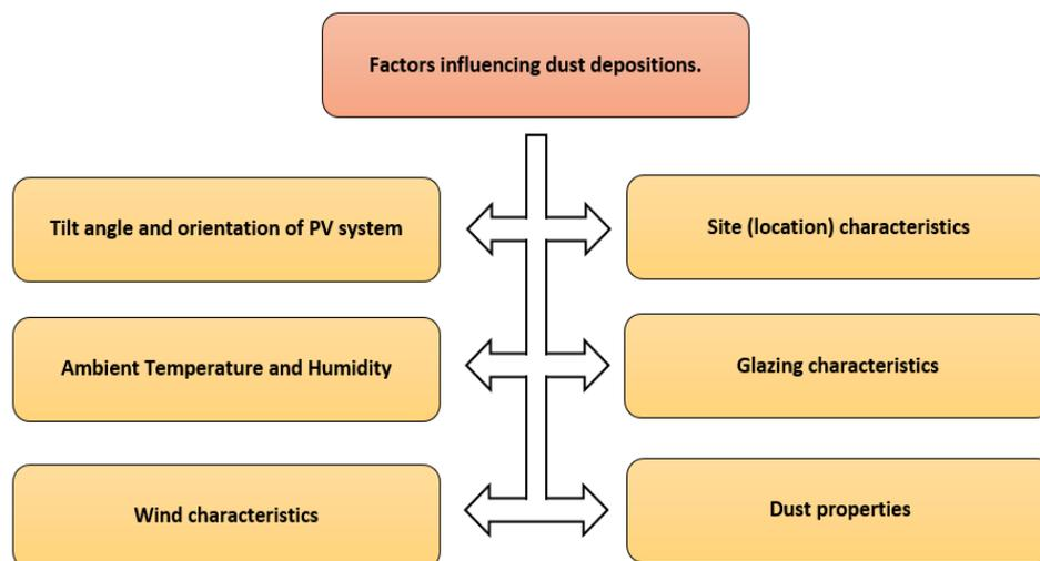
**Figure 1.** Factors influencing dust depositions on the surface of PV panels.
