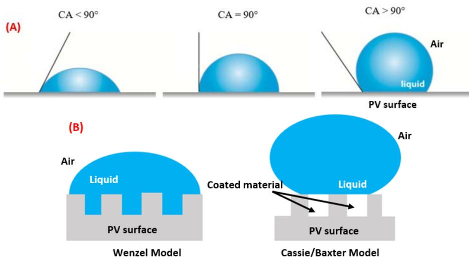
**Figure 4.** Behavior of a water droplet on a hydrophobic surface. (A) Water contact angles (CA) and (B) Wenzel and Cassie/Baxter models.
