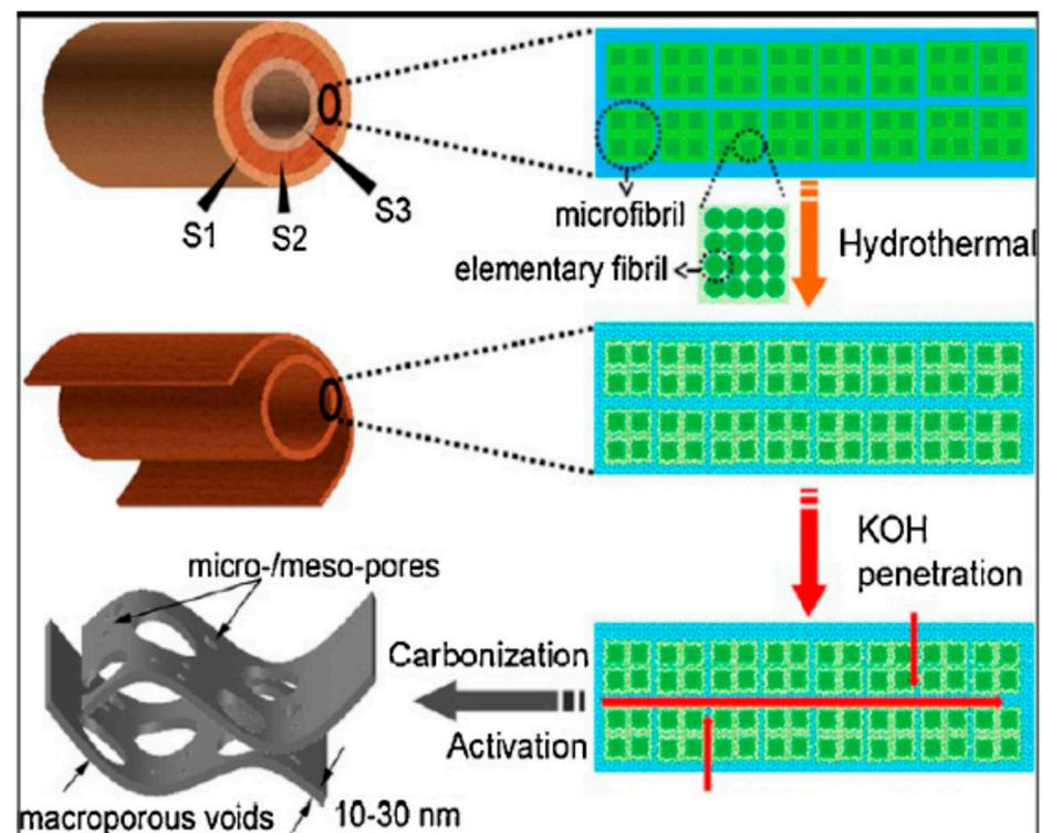
Figure 4. Preparation of graphene from Hemp fiber Reprinted with permission from ref. [39] Copyright 2013 American Chemical Society.
