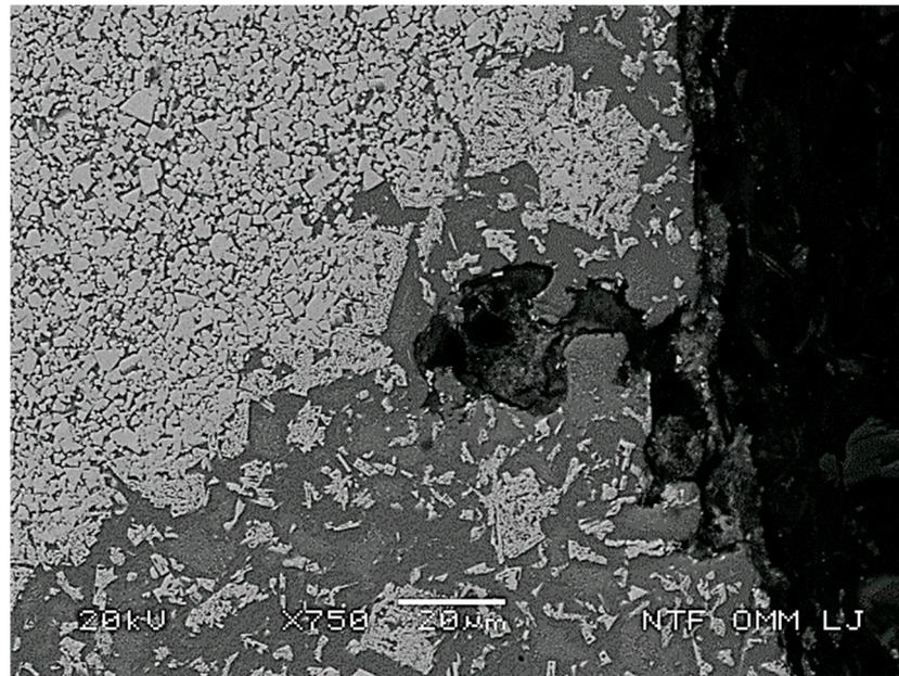
**Figure 13.** Formation of micro erosion channels in carbide coating matrix.
