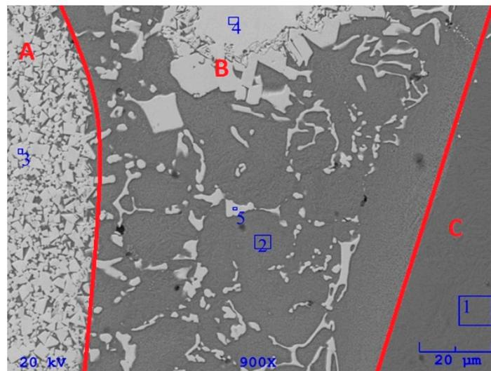
**Figure 6.** Tooth SEM image: 1—substrate (tooth base steel), 2—matrix of WC coating in transition zone, 3—WC, 4—WC in transition zone, 5—WC in transition zone, Zones: A—coating, B—transition zone (mixing zone), C—substrate (tooth body).
