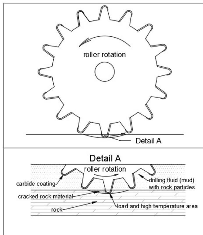
Figure 2. The action of the bit tooth on the rock.
