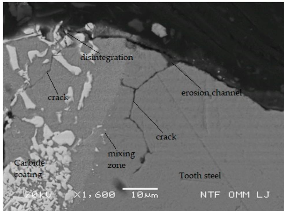
**Figure 11.** Formation of microcracks due to different elastic properties of materials.
