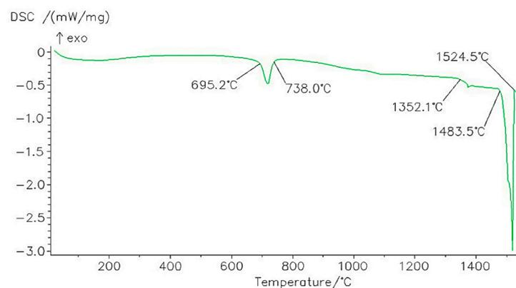
**Figure 7.** Heating curve of the tooth body steel.
