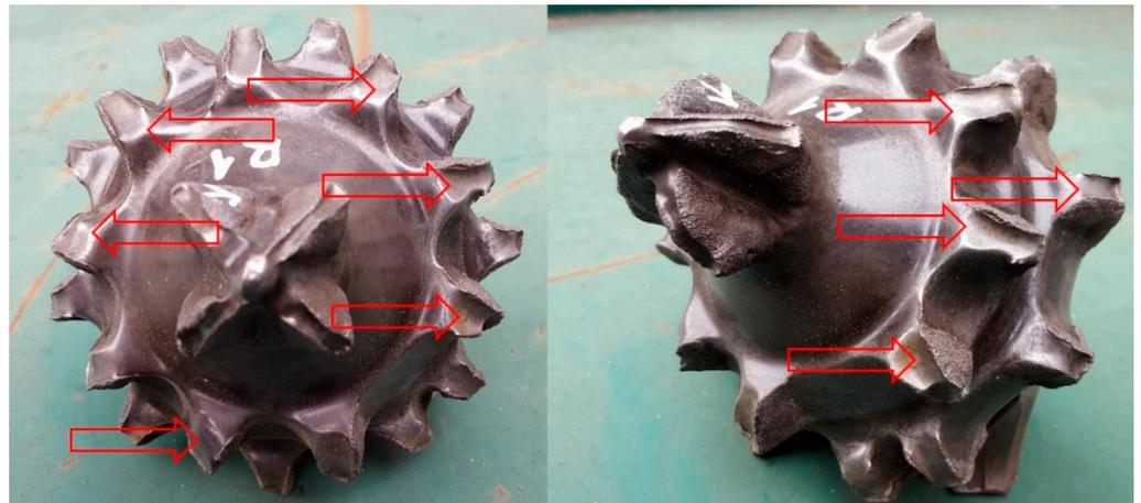
**Figure 10.** Characteristic wear of the teeth of the roller cone bit.
