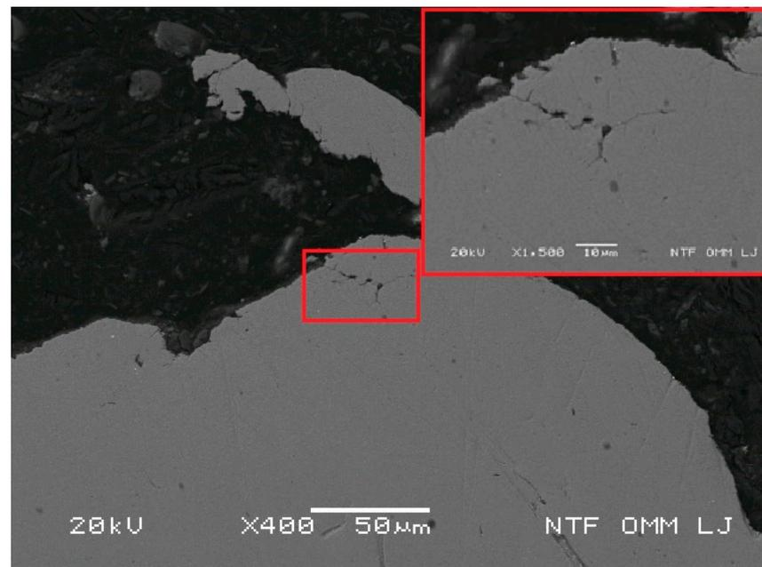
**Figure 12.** Micro cracks and erosion channels.
