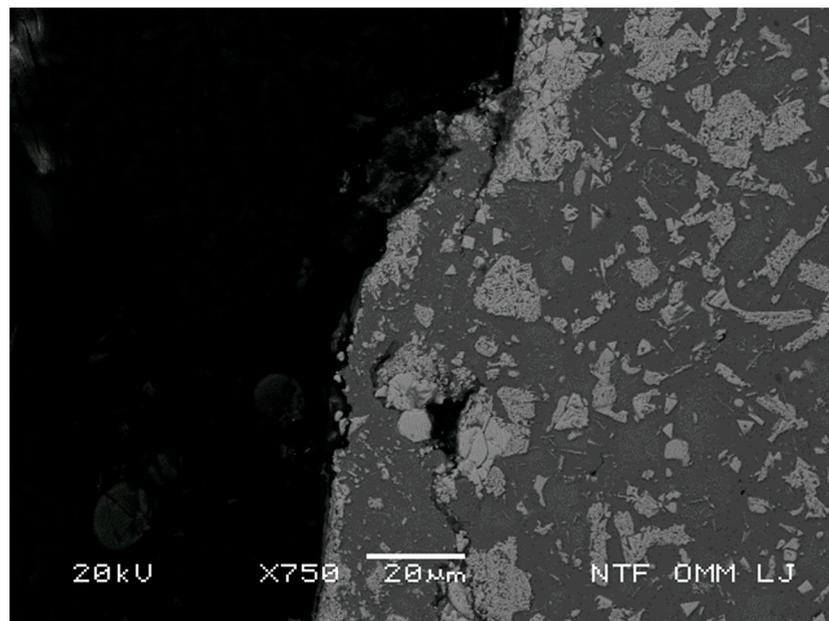
**Figure 14.** Formation of micro erosion channels in carbide coating matrix.
