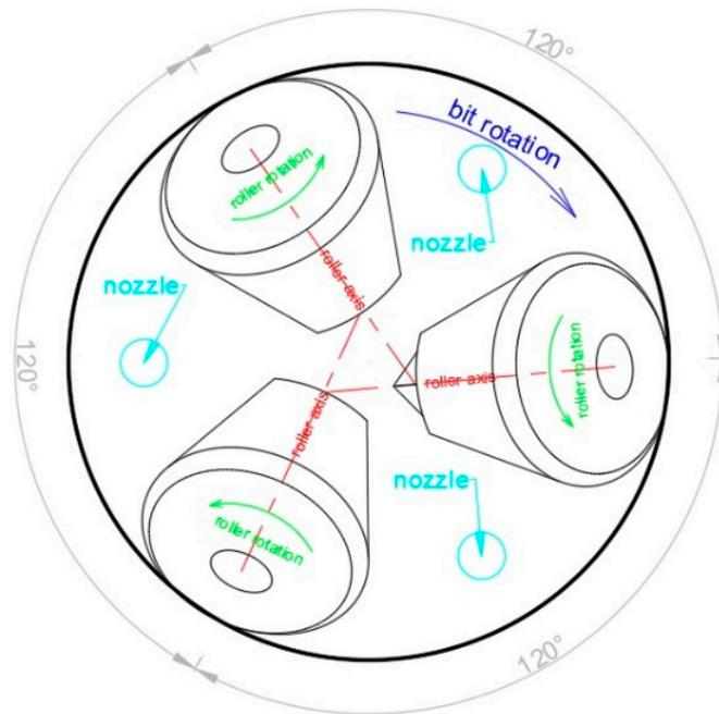
Figure 1. Settings of rollers for soft rock formations roller cone drill bits.
