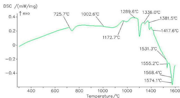
**Figure 8.** Heating curve of the carbide coating.
