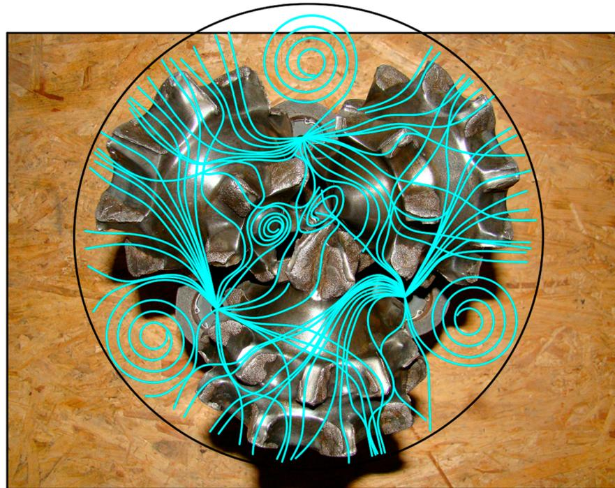
**Figure 3.** Simplified sketch of the movement of the drilling fluid in the area of the rollers.
