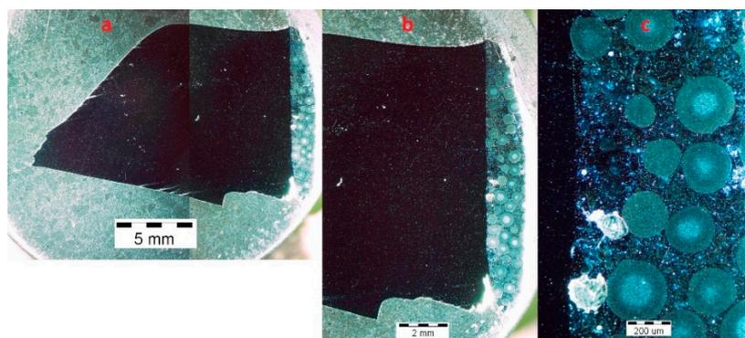
**Figure 5.** Cross section of a worn tooth with a protective carbide coating.
