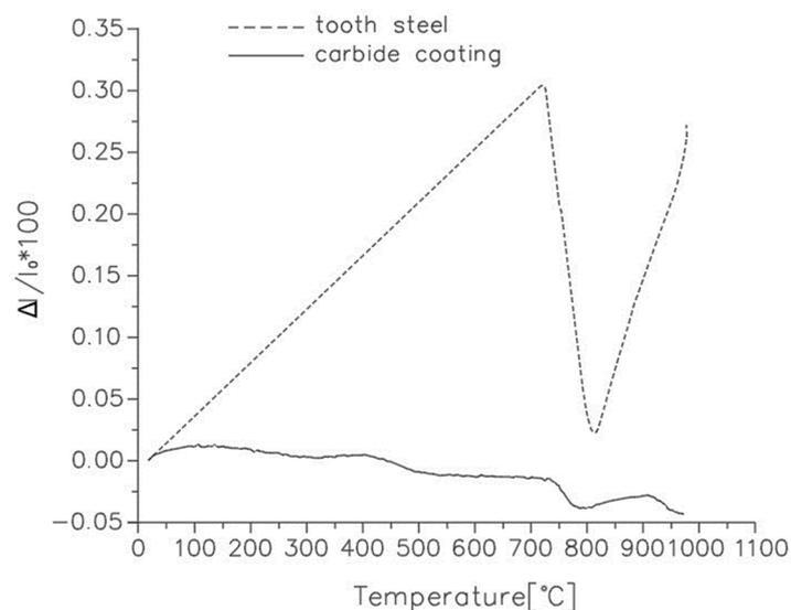
**Figure 9.** Dilatometric curves of the substrate steel and the coating.
