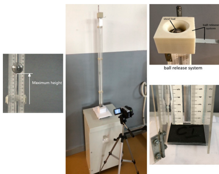
Figure 4. Shock impact device: impact testing experimental setup.
