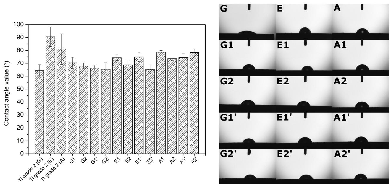
**Figure 6.** The results of the water contact angle measurements for the surface of pre-treated Ti grade 2 substrates and the modified substrates with chit/EE100 coatings obtained for different process parameters. Data are presented as the mean  $\pm$  SD (n = 5).
