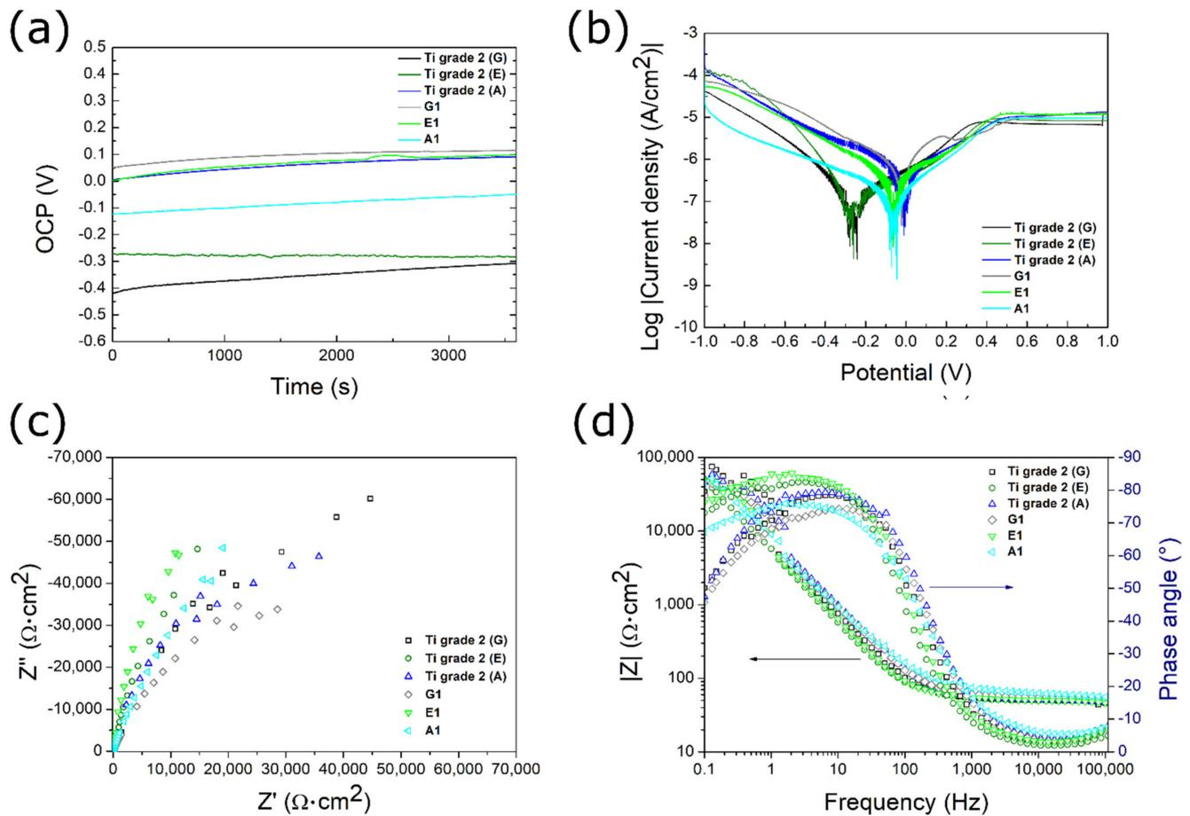
**Figure 8.** (a) Open circuit potential (OCP); (b) potentiodynamic polarization curves; (c) Nyquist plots; and (d) Bode plots of the surface of pre-treated Ti grade 2 substrates and samples with chit/EE100 coatings.
