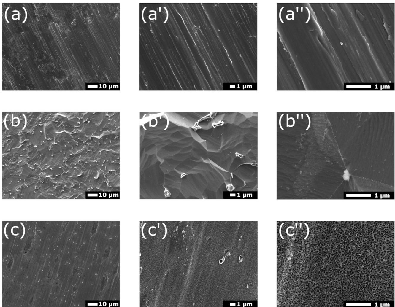
**Figure 1.** SEM images of surface pretreated Ti grade 2 substrates after (a) wet grinding, (b) acid etching, and (c) electrochemical anodization in different magnifications:  $\times 1000$  (a–c),  $\times 5000$  (a'–c'), and  $\times 25000$  (a''–c'').
