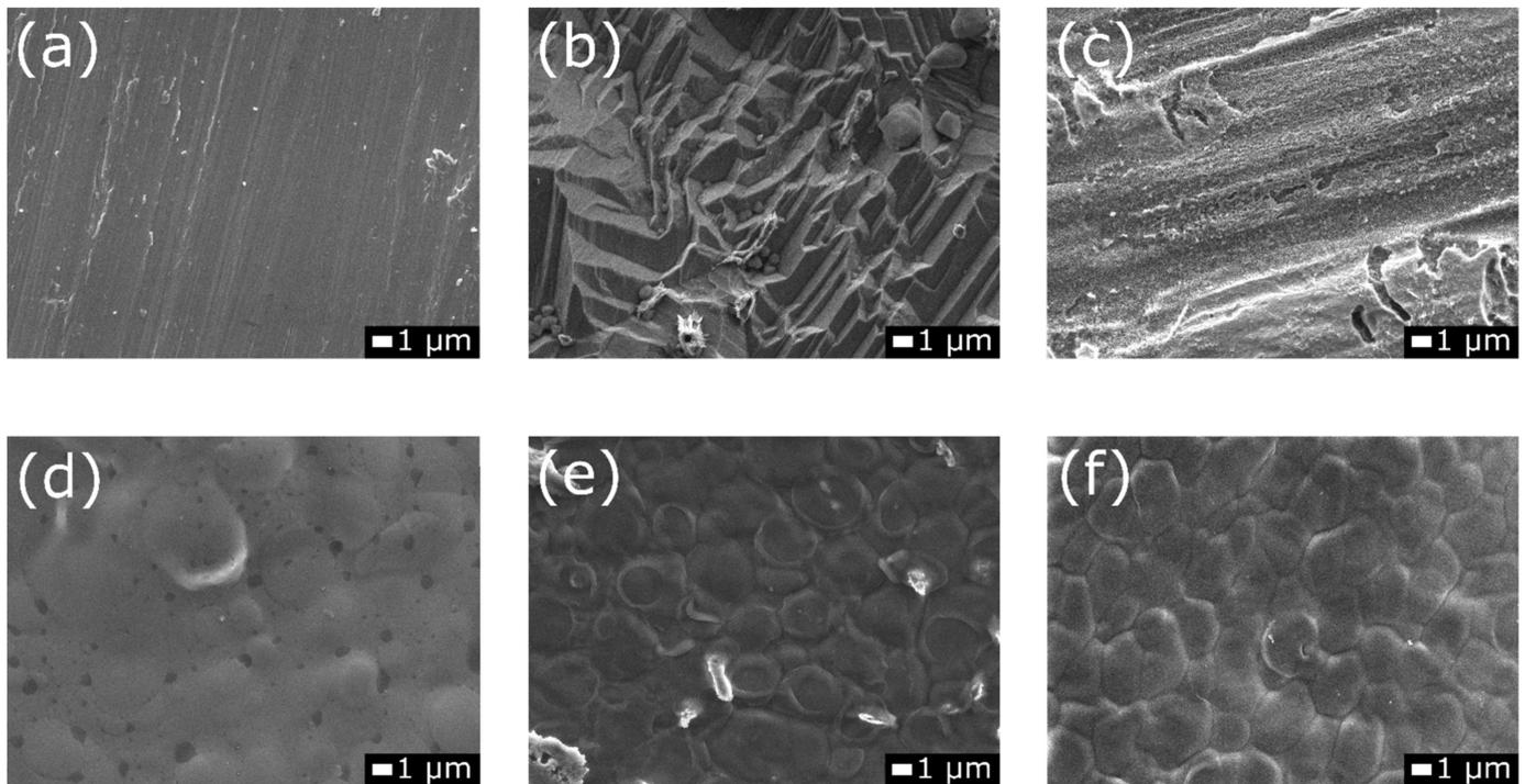
**Figure 9.** SEM images of the surface of pre-treated Ti grade 2 substrates after (a) wet grinding (G), (b) acid etching (E), and (c) electrochemical anodization (A), and for the samples: (d) G1, (e) E1, and (f) A1 with chit/EE100 coatings after electrochemical tests (images obtained with magnification at  $\times 5000$ ).
