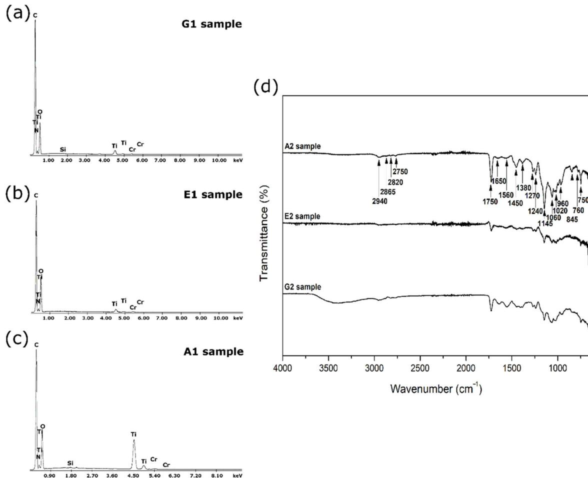
**Figure 5.** EDS (a), (b), (c), and FTIR (d) analysis results of samples with chit/EE100 coatings deposited on substrates after (a) grinding (sample G1), (b) etching (sample E1), and (c) electrochemical oxidation (sample A1).
