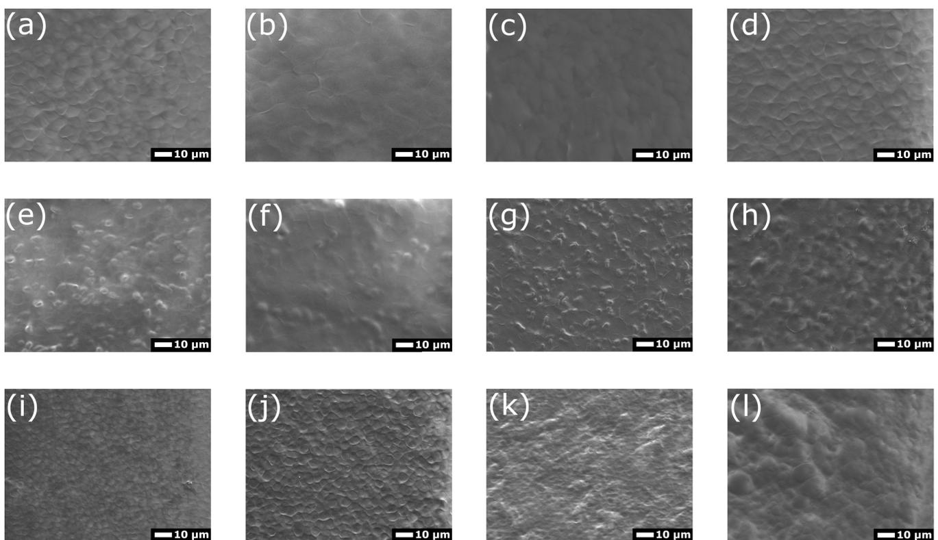
**Figure 3.** SEM images of chitosan/EE100 coatings deposited on the surface of pre-treated Ti grade 2 samples for different process parameters: (a) G1, (b) G2, (c) G1', (d) G2', (e) E1, (f) E2, (g) E1', (h) E2', (i) A1, (j) A2, (k) A1', and (l) A2' sample, magnification  $\times 1000$ .
