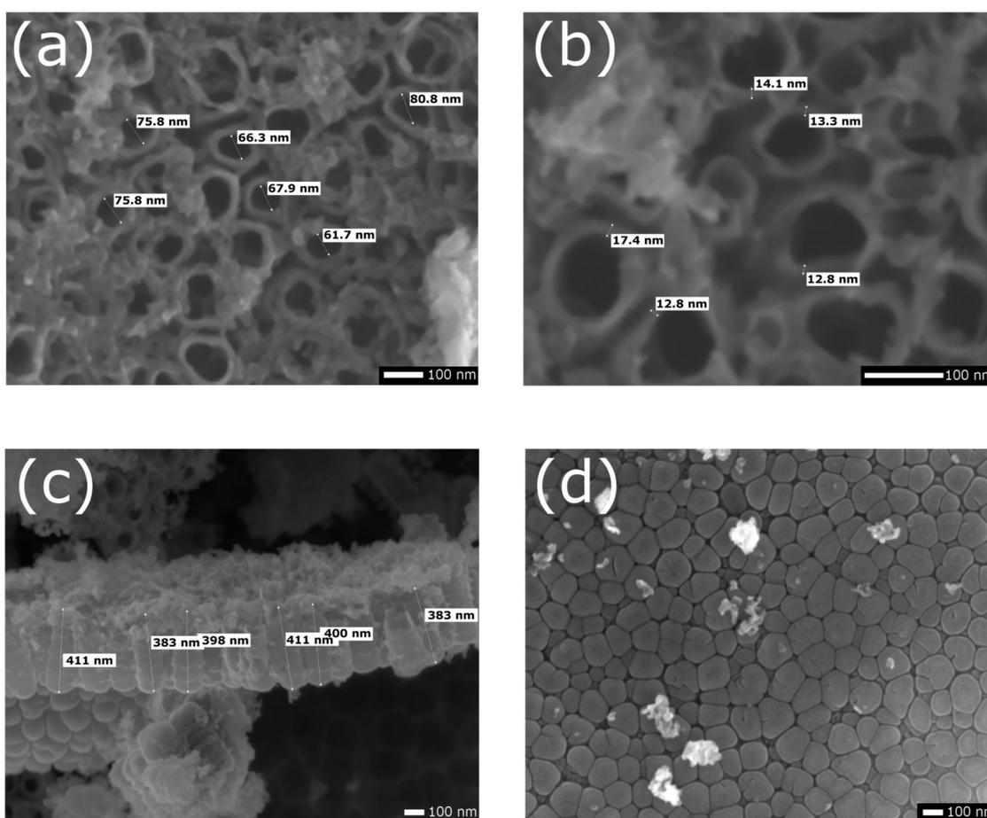
**Figure 2.** SEM images of TiO<sub>2</sub> nanotubes on titanium grade 2 obtained by electrochemical anodization at 20 V for 20 min: (a) top view with inner diameter measurements of nanotubes; (b) top view with nanotube wall thickness measurements; (c) cross-sectional view with nanotube length measurements; and (d) bottom view of nanotubes.
