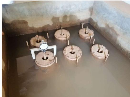
Figure 4. CBR swell tripod for measuring swell.
