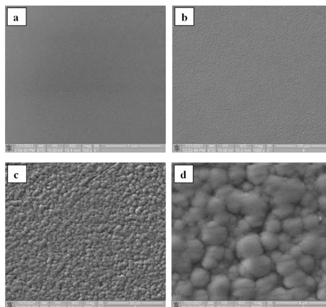
**Figure 34.** Micrographs of the obtained coatings at various magnifications: (a) 500×, (b) 1000×, (c) 5000×, (d) 25,000×.
