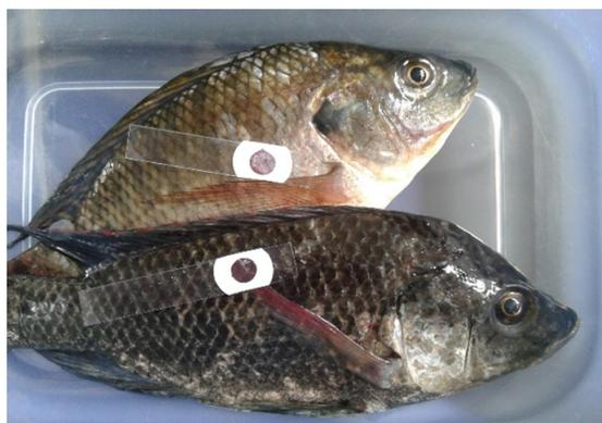
**Figure 1.** The fabricated sensors were attached onto the skin of the fish to detect the pH changes before the absorbance was measured with a UV-Vis spectrophotometer.
