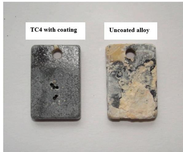
**Figure 3.** Macrophotograph of TC4 with and without coating after corrosion in marine environment for 100 h at 650 °C.
