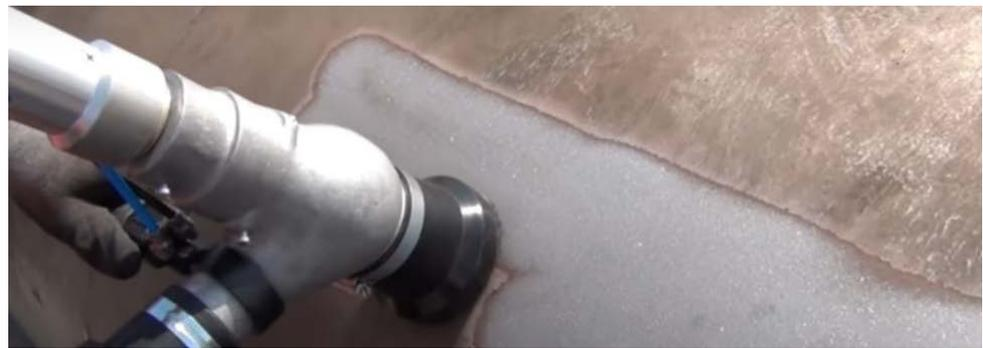
**Figure 4.** The process of shot blasting the surface of the hydraulic cylinder rod.
