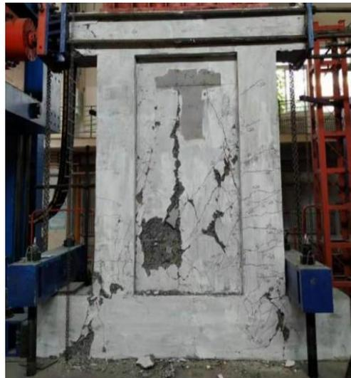
**Figure 7.** Final damage of specimen XJ.
