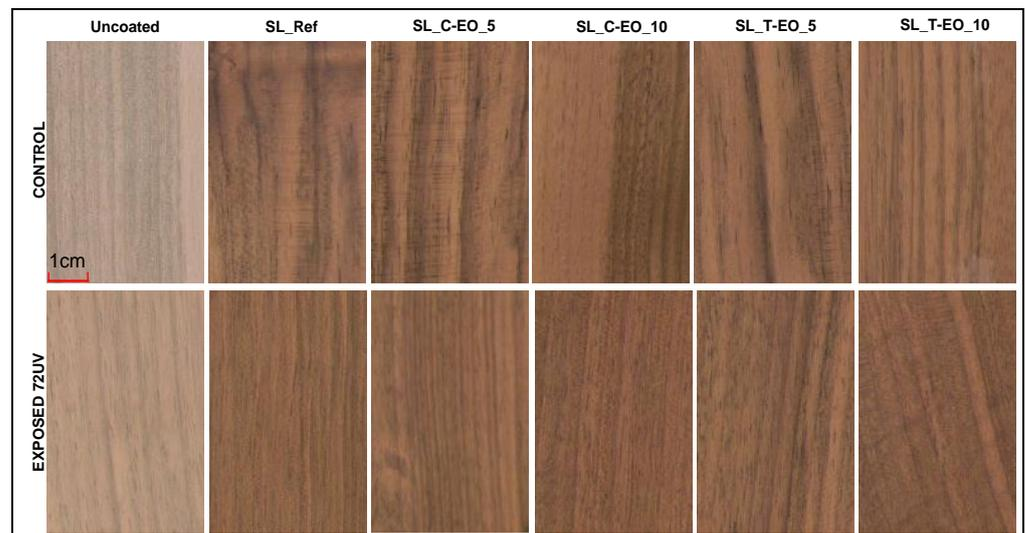
**Figure 5.** Images illustrating the aspect of walnut (*Juglans regia*) wood samples before and after coating with the five different types of shellac solutions: control samples before ageing and aged samples after 72 h UV exposure.
