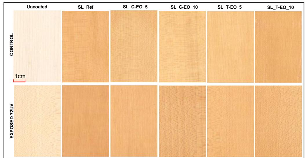
**Figure 4.** Images illustrating the aspect of maple (*Acer pseudoplatanus*) wood samples before and after coating with the five different types of shellac solutions: control samples before ageing and aged samples after 72 h UV exposure.
