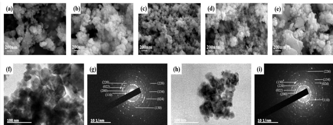
**Figure 2.** SEM images of (a)  $\text{LaMnO}_3$ , (b)  $\text{La}_{0.95}\text{Sr}_{0.05}\text{MnO}_3$ , (c)  $\text{La}_{0.9}\text{Sr}_{0.1}\text{MnO}_3$ , (d)  $\text{La}_{0.85}\text{Sr}_{0.15}\text{MnO}_3$ , and (e)  $\text{La}_{0.8}\text{Sr}_{0.2}\text{MnO}_3$ ; (f,g) TEM image and selected area electron diffraction images of  $\text{LaMnO}_3$ ; (h,i) TEM image and selected area electron diffraction patterns of  $\text{La}_{0.85}\text{Sr}_{0.15}\text{MnO}_3$ .
