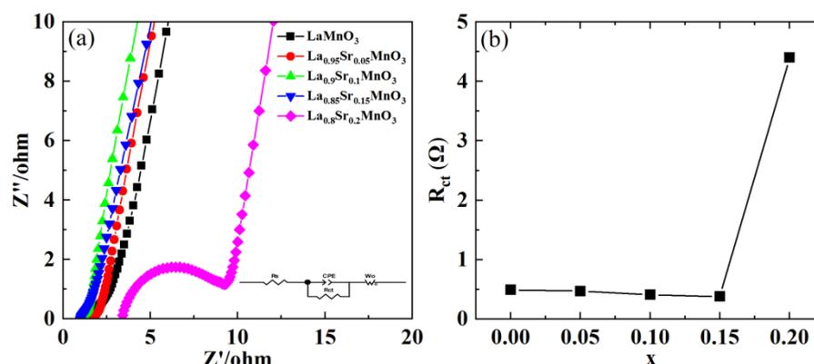
**Figure 7.** (a) The impedance comparison diagram of  $\text{La}_{1-x}\text{Sr}_x\text{MnO}_3$  ( $x = 0.0, 0.05, 0.1, 0.15$ , and  $0.2$ ) electrodes; (b) The  $R_{ct}$  of  $\text{La}_{1-x}\text{Sr}_x\text{MnO}_3$  ( $x = 0.0, 0.05, 0.1, 0.15$ , and  $0.2$ ) electrodes.
