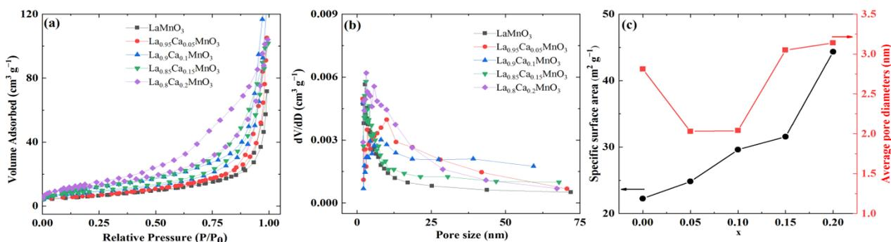
**Figure 3.** (a)  $\text{N}_2$  adsorption–desorption isotherms of  $\text{La}_{1-x}\text{Sr}_x\text{MnO}_3$  ( $x = 0.0, 0.05, 0.1, 0.15,$  and  $0.2$ ) nanoparticles, (b) BJH pore size distributions of  $\text{La}_{1-x}\text{Sr}_x\text{MnO}_3$  ( $x = 0.0, 0.05, 0.1, 0.15,$  and  $0.2$ ) nanoparticles, (c) The specific surface area and average pore diameters of  $\text{La}_{1-x}\text{Sr}_x\text{MnO}_3$  ( $x = 0.0, 0.05, 0.1, 0.15,$  and  $0.2$ ).
