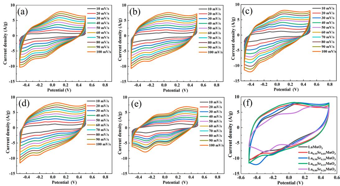
**Figure 5.** CV curves of  $\text{La}_{1-x}\text{Sr}_x\text{MnO}_3$  ( $x = 0.0, 0.05, 0.1, 0.15, \text{ and } 0.2$ ): (a)  $\text{LaMnO}_3$ ; (b)  $\text{La}_{0.95}\text{Sr}_{0.05}\text{MnO}_3$ ; (c)  $\text{La}_{0.9}\text{Sr}_{0.1}\text{MnO}_3$ ; (d)  $\text{La}_{0.85}\text{Sr}_{0.15}\text{MnO}_3$ ; (e)  $\text{La}_{0.8}\text{Sr}_{0.2}\text{MnO}_3$ ; (f) CVs recorded at a scan rate of 100 mV/s for all samples in 3 M KOH electrolyte.
