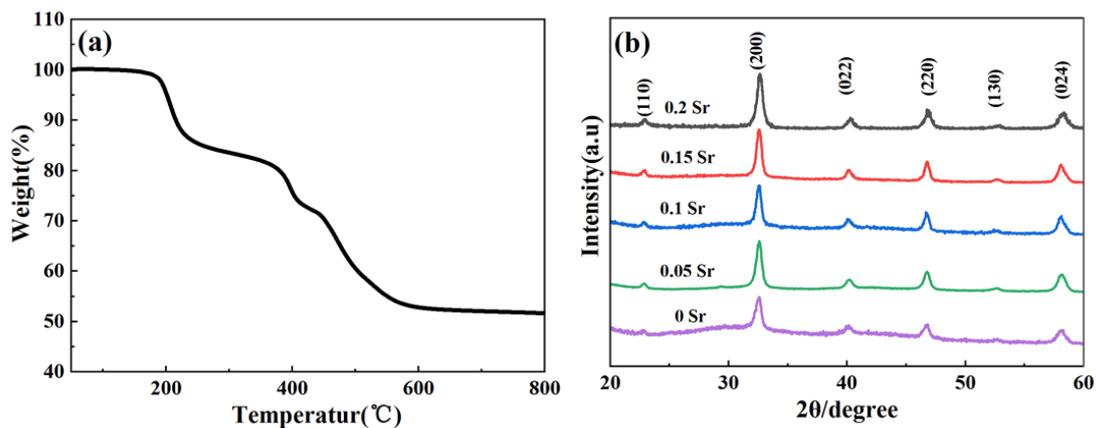
**Figure 1.** (a) TG curve of the  $\text{LaMnO}_3$  precursor and (b) XRD pattern of  $\text{La}_{1-x}\text{Sr}_x\text{MnO}_3$  ( $x = 0.0, 0.05, 0.1, 0.15,$  and  $0.2$ ).
