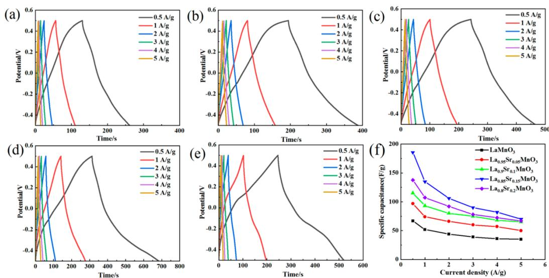
**Figure 6.** Charge–discharge curves of  $\text{La}_{1-x}\text{Sr}_x\text{MnO}_3$  ( $x = 0.0, 0.05, 0.1, 0.15,$  and  $0.2$ ): (a)  $\text{LaMnO}_3$ ; (b)  $\text{La}_{0.95}\text{Sr}_{0.05}\text{MnO}_3$ ; (c)  $\text{La}_{0.9}\text{Sr}_{0.1}\text{MnO}_3$ ; (d)  $\text{La}_{0.85}\text{Sr}_{0.15}\text{MnO}_3$ ; (e)  $\text{La}_{0.8}\text{Sr}_{0.2}\text{MnO}_3$ ; and (f) specific current against the specific capacitance of  $\text{La}_{1-x}\text{Sr}_x\text{MnO}_3$ .
