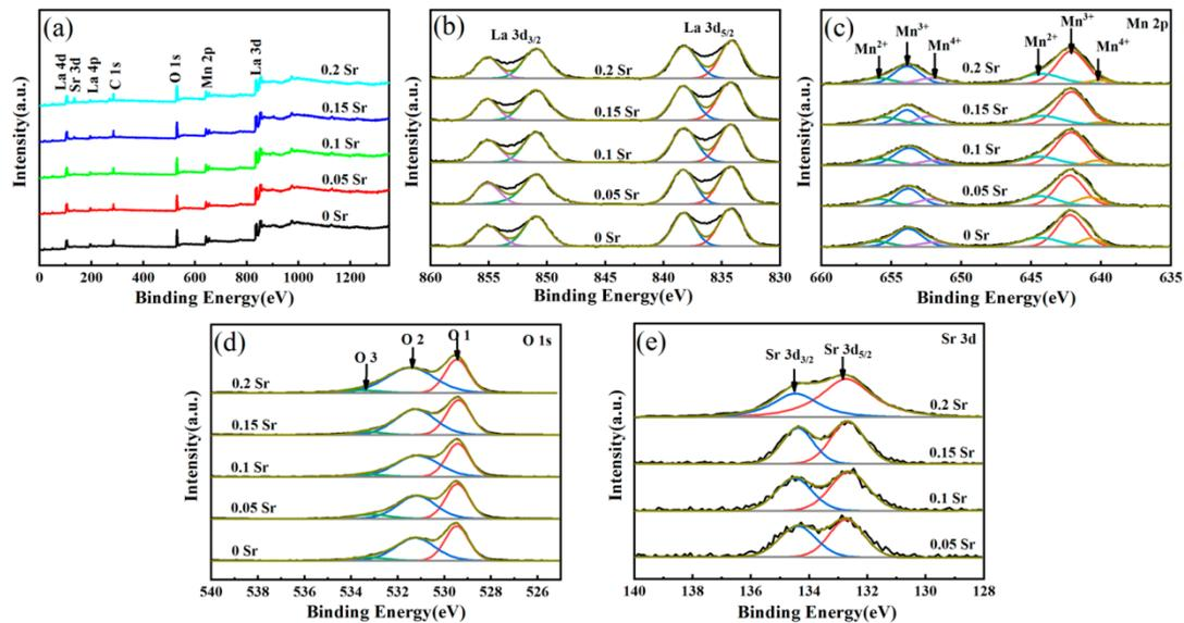
**Figure 4.** (a) XPS survey spectrum of  $\text{La}_{1-x}\text{Sr}_x\text{MnO}_3$  ( $x = 0.0, 0.05, 0.1, 0.15,$  and  $0.2$ ); high-resolution spectrum of (b) La3d, (c) Mn2p, (d) O1s, and (e) Sr3d.
