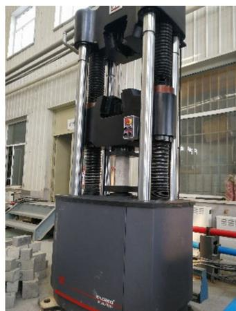
**Figure 5.** Loading equipment of electro-hydraulic servo universal testing machine.
