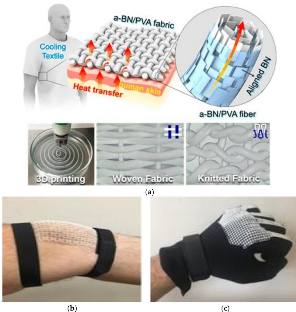
**Figure 2.** (a) Schematic illustration of the thermal regulation textile made with 3D printing [61]. Copyright 2017, American Chemical Society. (b) A mesh, featuring anisotropic mechanics and showing the ability to conform to a knee. (c) The mesh is sewn onto a glove and this mesh-enhanced glove exerts a restoring force on the fingers when the fist is clenched [62]. Copyright 2019, Wiley-VCH.
