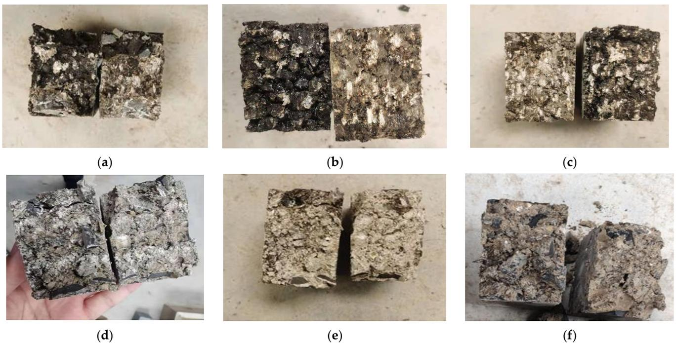
**Figure 7.** Shear failure form of specimens without interlaminar treatment. (a) I-1; (b) I-2; (c) I-3; (d) I-5; (e) I-6; (f) I-7.
