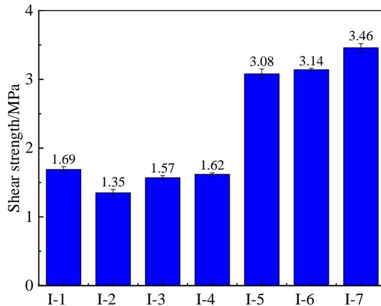
Figure 6. Shear strength of specimens without interlaminar treatment.
