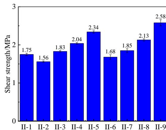
**Figure 8.** Shear strength of specimens.
